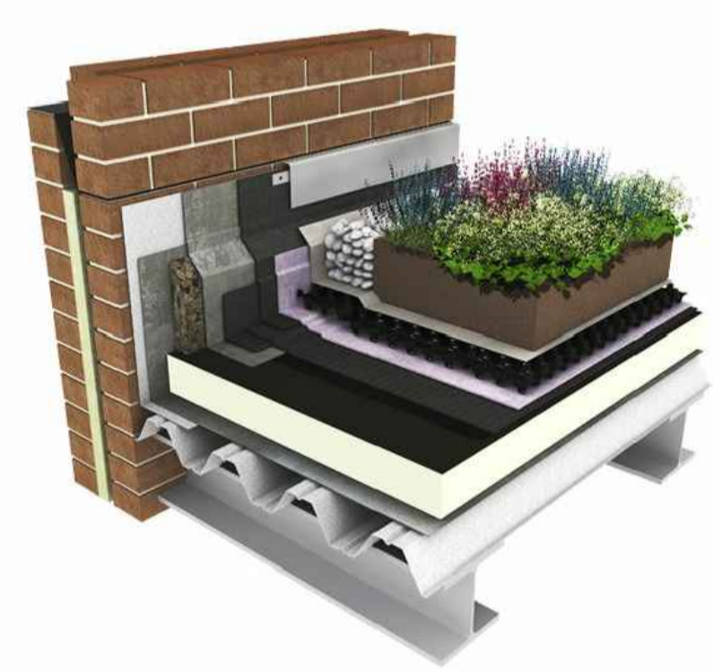
00 Typical extensive biodiverse green roof system Scale: nts
