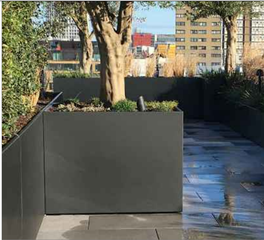
F13 Bespoke Movable Planter MANUFACTURER: Kinley RANGE: 1000(w) x 1000(d) x 1000(h)mm WEBSITE: www.kinley.co.uk MATERIAL: Mild steel powder coated to RAL 7016 FIXING: Freestanding/ with lockable casters to base of planter to allow planters to be manually moveable. skirt required around the edge of planter to hide wheels
