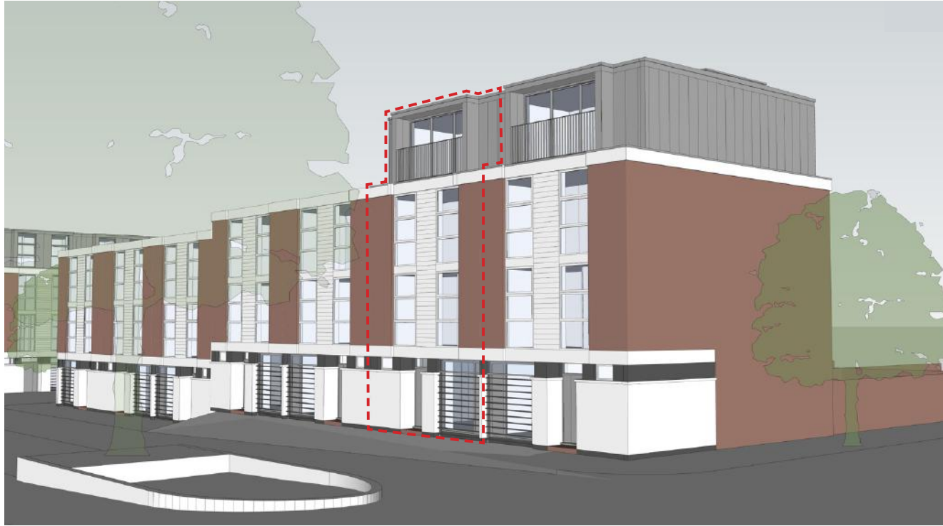
Proposed front (east) elevation of extension to No 38 (highlighted), with the approved extension for No 39.
