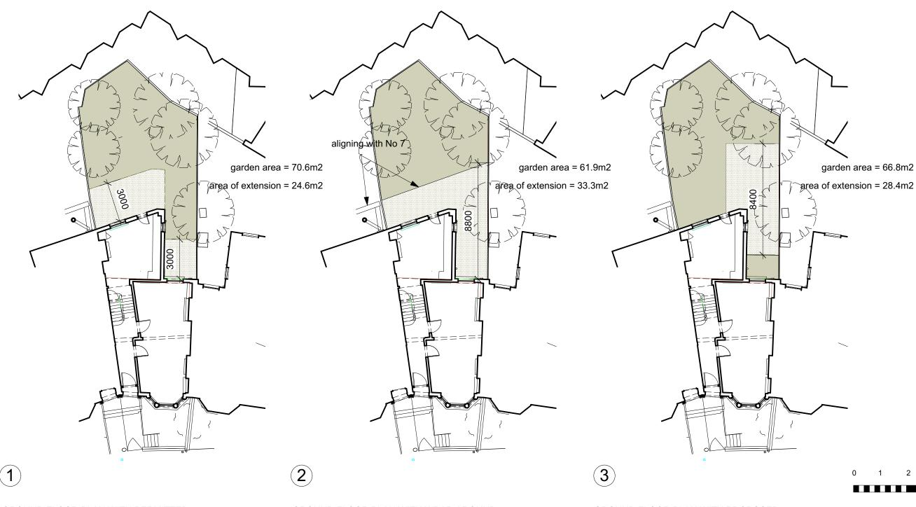
GROUND FLOOR PLAN WITH PERMITTED DEVELOPMENT SHOWN scale 1:200
