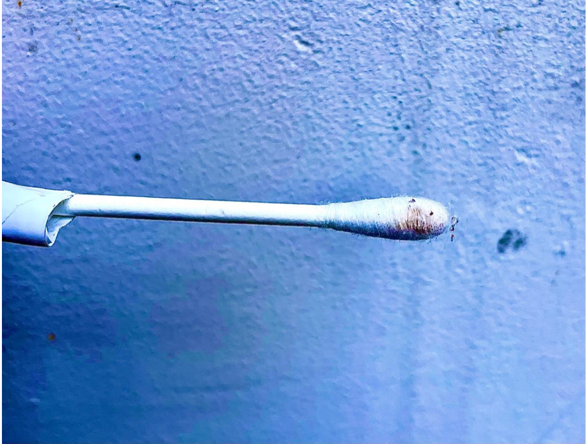
Cotton sample showing metal oxidized flecks from interior brick surround
