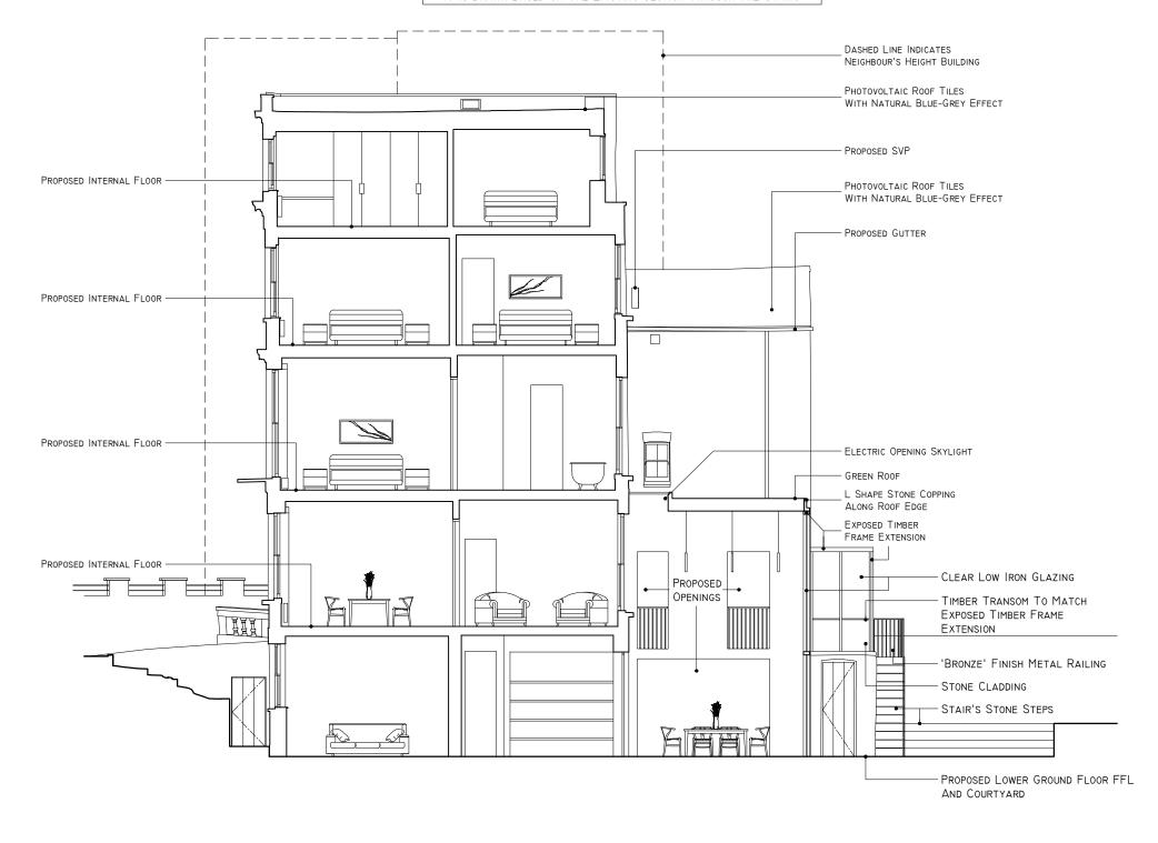
PROPOSED EAST ELEVATION & SECTION
