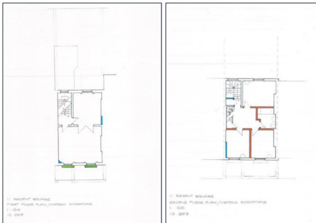
Images 10-11: Existing first-floor and second-floor plans indicating the age of existing alterations
