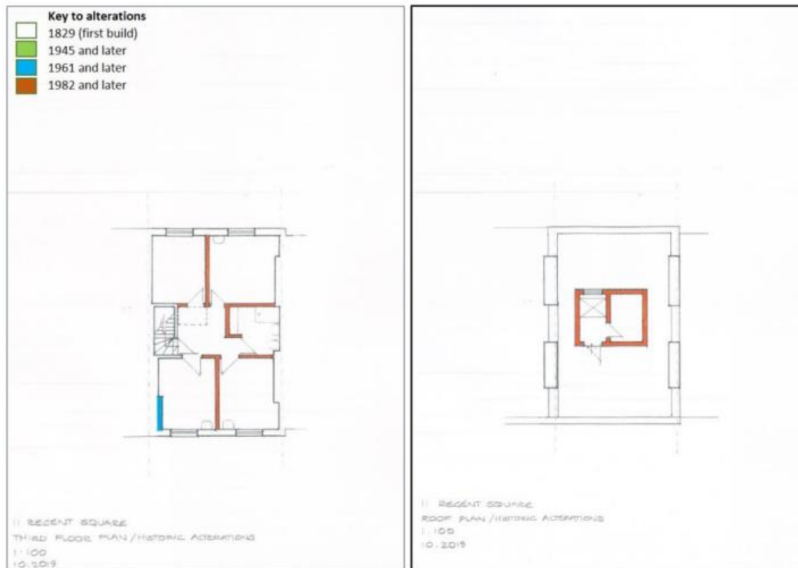
Images 12-13: Existing third-floor and roof plans indicating the age of the existing alterations
