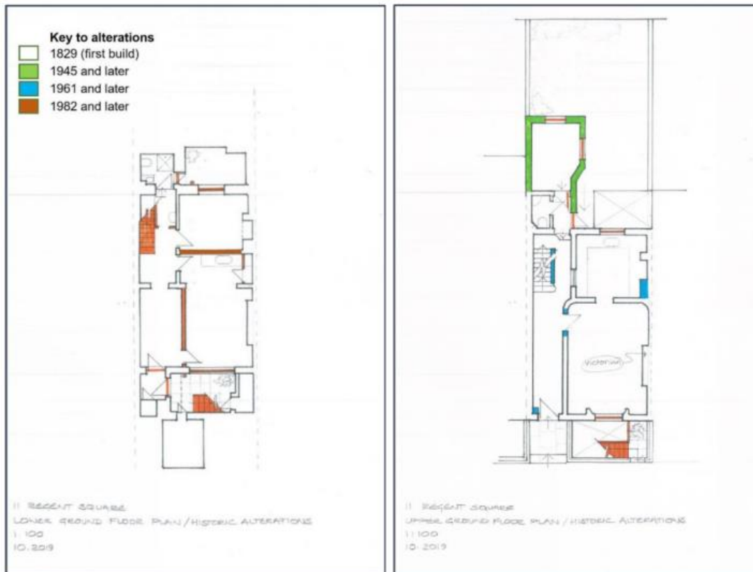
Images 8-9: Existing lower ground floor and upper ground floor plans indicating the age of existing alterations
