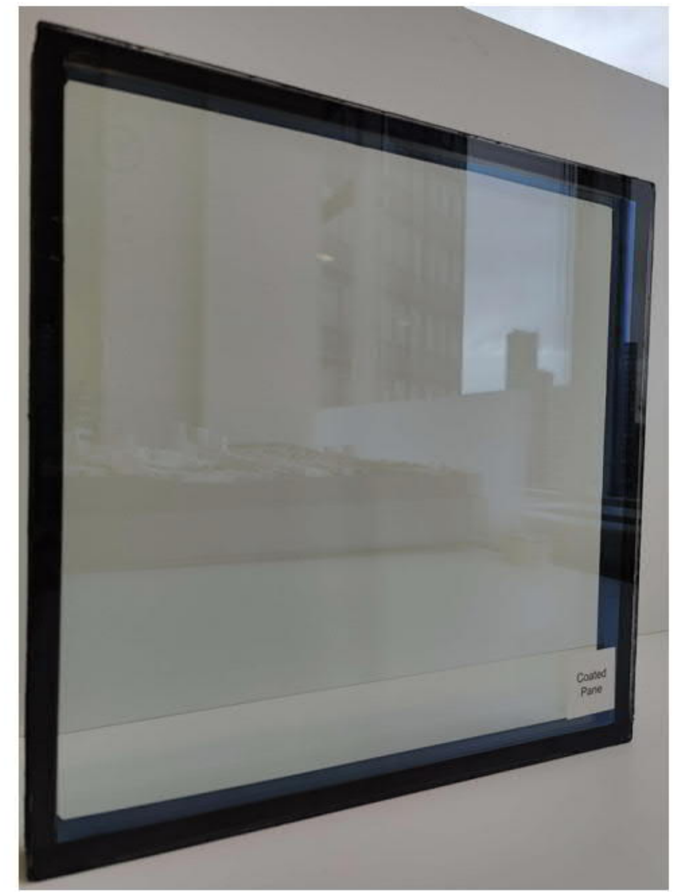
double glazed unit (8.8mm laminated outer pane, 16mm argon filled cavity, 6mm toughened inner pane)
