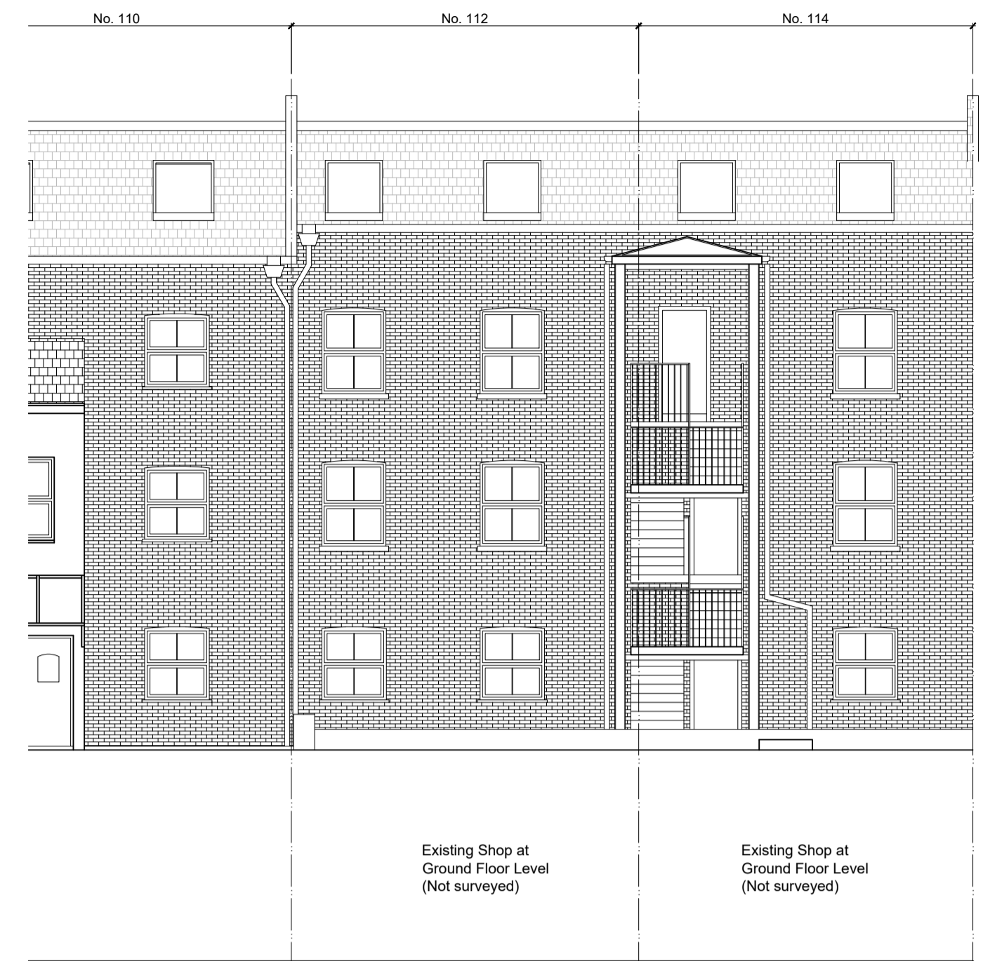
Existing Rear (North-East) Elevation Scale 1:100
