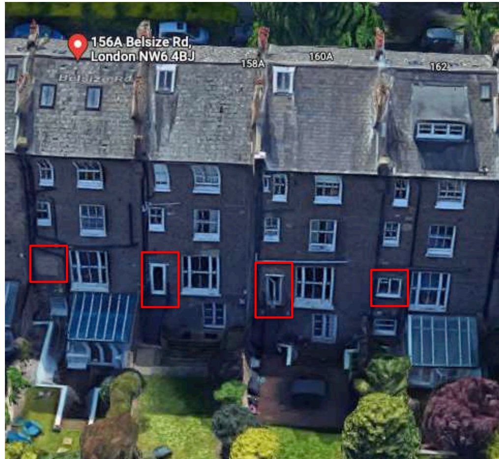
Aerial view of rear elevations to terrace showing secondary window/ door openings at first floor level
