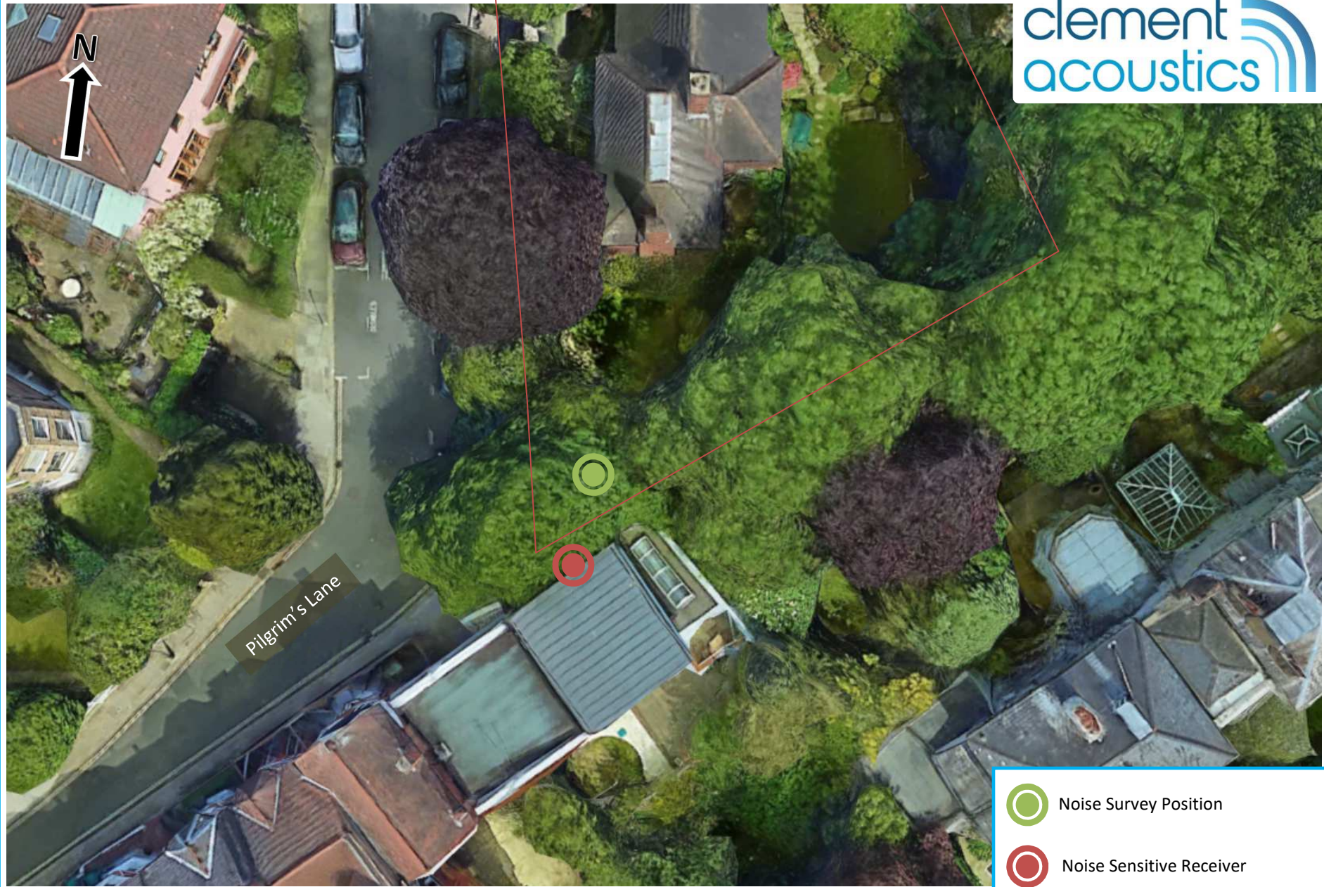
17451-SP1 Indicative site plan indicating noise monitoring position, nearest noise sensitive receiver and proposed plant location
