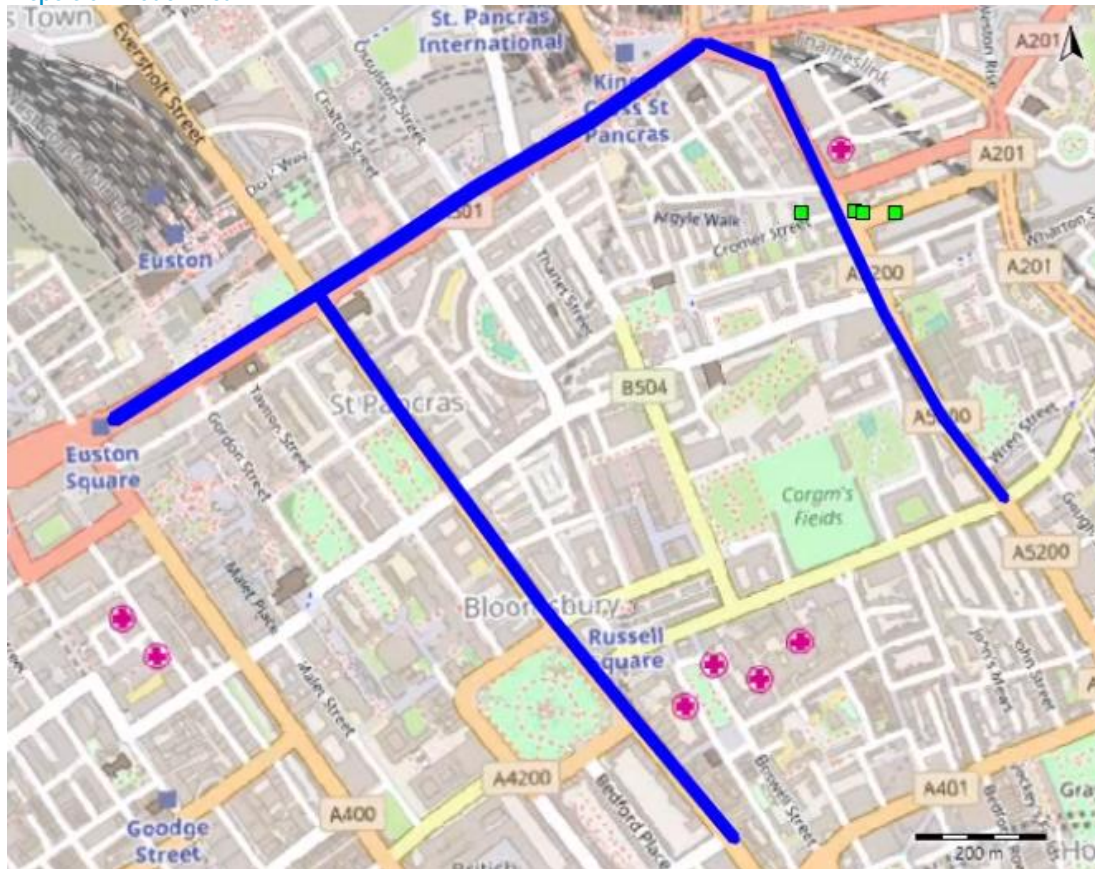
Figure D- 1: Dispersion model area, showing road emissions sources (in blue) and modelled receptors around the development (in green).
