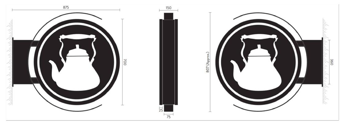
**Projection Signage:** Fabricated projection signage consisting of fabricated 3mm shaped rim/return aluminium panels 700mm diameter x 150mm deep overall. Coated RAL 9005 black satin. 5mm opal acrylic faces with vinyl decorations applied (black background with white vinyl graphics), illuminated internally with white LEDs (cd/m<sup>2</sup>: 600 - static illumination). Completed with wall brackets and shroud, coated RAL 9005 black satin.
