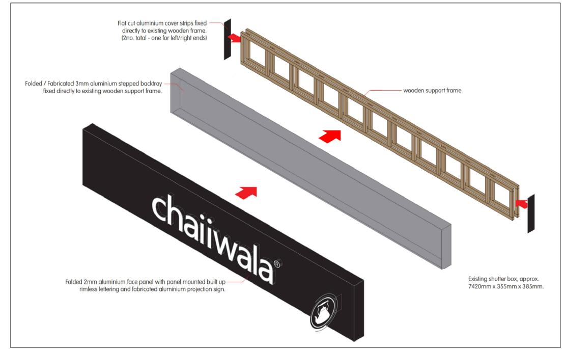
**Illuminated Fascia Signage:** Folded 3mm aluminium panel, 70mm deep, coated RAL 9005 black satin. Folded 3mm aluminium backtray to suit. Coated RAL 9005 black satin externally. Panel mounted built up rimless letters to read "Chaiiwala", Internally illuminated with white LEDs. Coated RAL 9005 black satin. 5mm opal 050 acrylic faces and 10mm white fomex backtrays (Black background with illuminated letters (cd/m<sup>2</sup>: 600 - static illumination).
