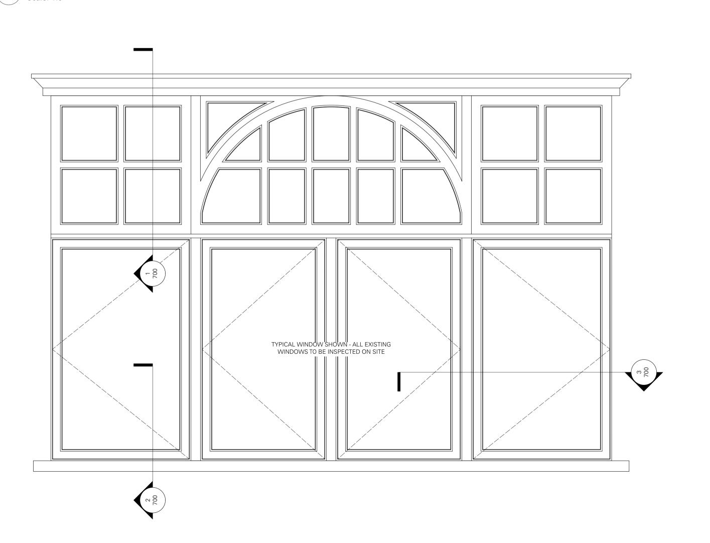
**TYPICAL EXISTING WINDOW - ELEVATION** Scale: 1:10
