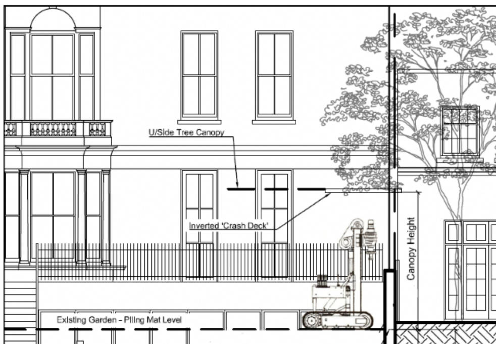
Fig. 2 Inverted Crash Deck Tree Protection Barrier Specification (N.b. there is no piling at this site)
