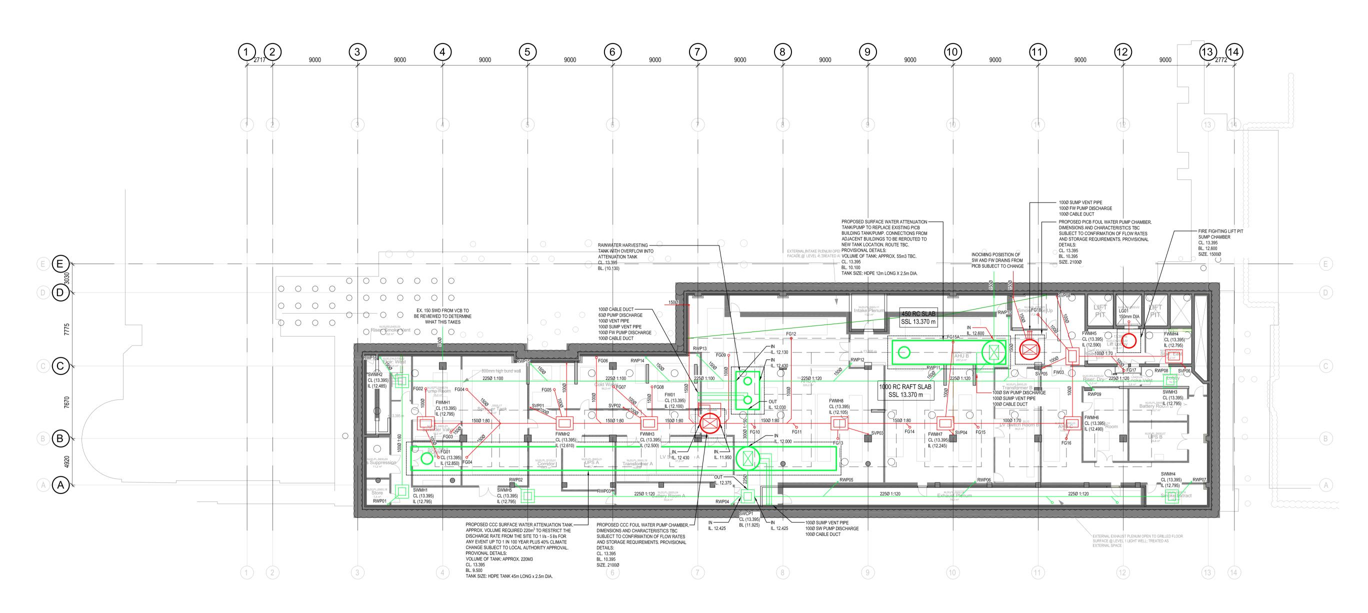
DRAIN CAVITY AND GULLIES/SUMPS
