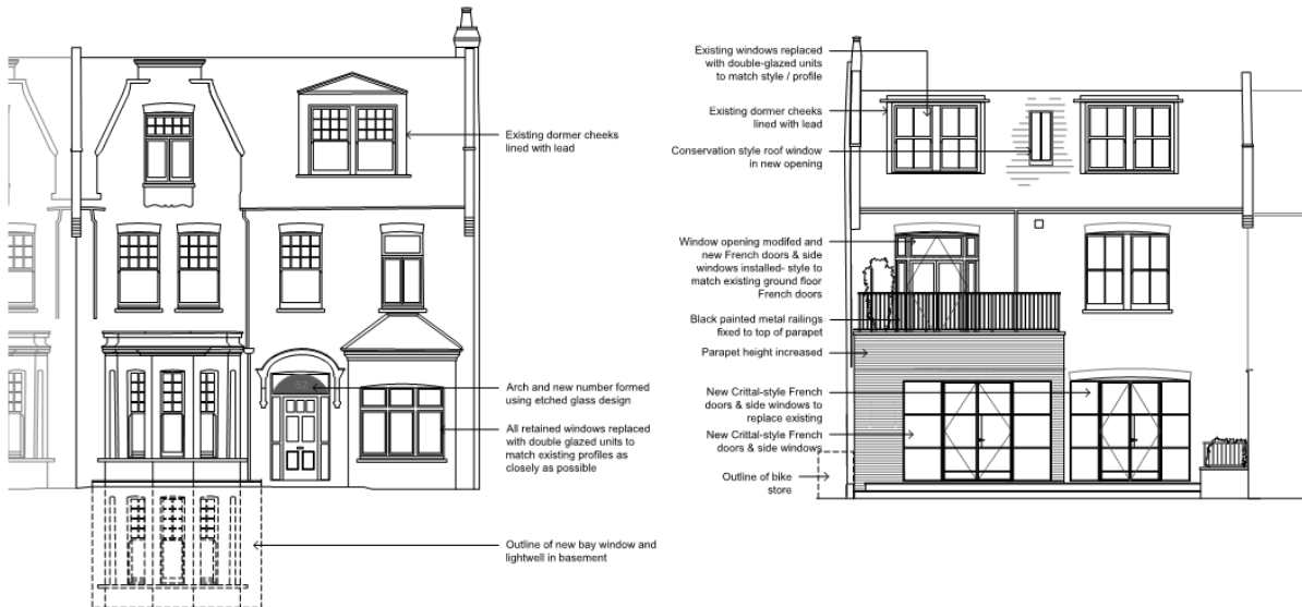
SOUTH WEST ELEVATION
