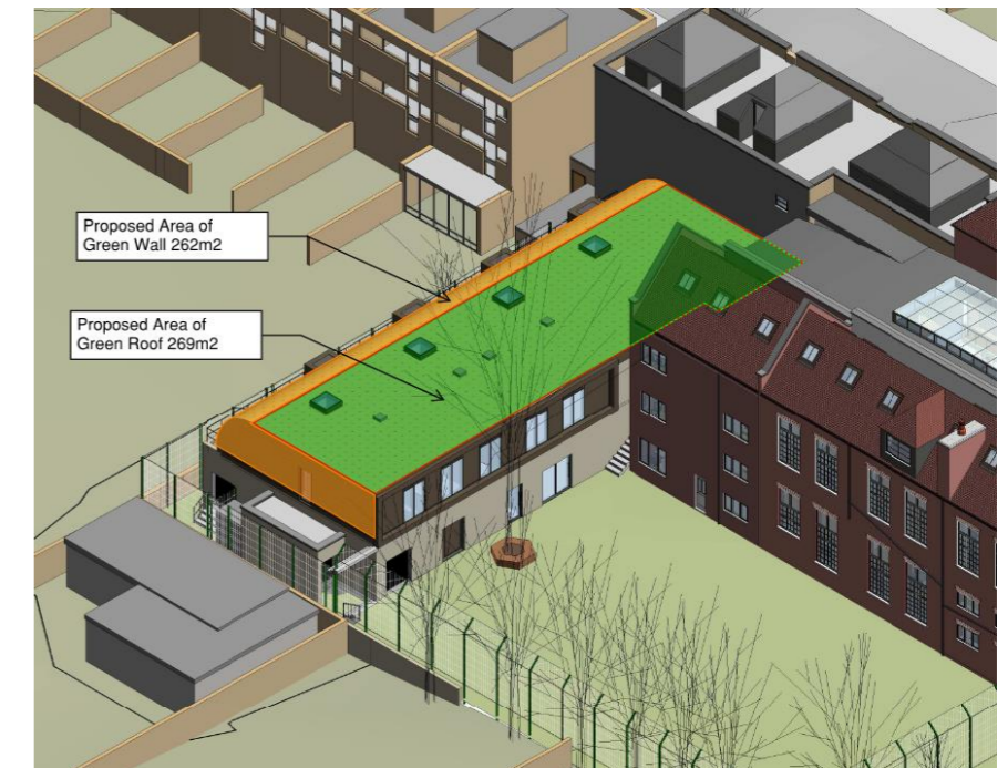
Figure 3 – Proposed green roof and green wall extents
