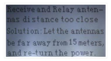
If the device detects that the outdoor antenna is too close to the indoor, change the position of either or both antennas to avoid self-oscillation. Mount them at least 15m one from another.
