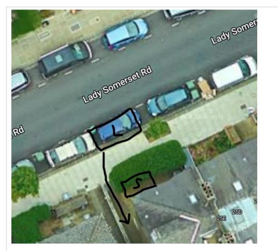
During the demolition phase a skip will be positioned in the front garden of the property (marked with S in the plan above). A skip lorry will lift the skip over the garden fence (which will be partly demolished and later rebuilt). If this is not possible or cannot be done safely the skip will be positioned on a suspended parking bay.
