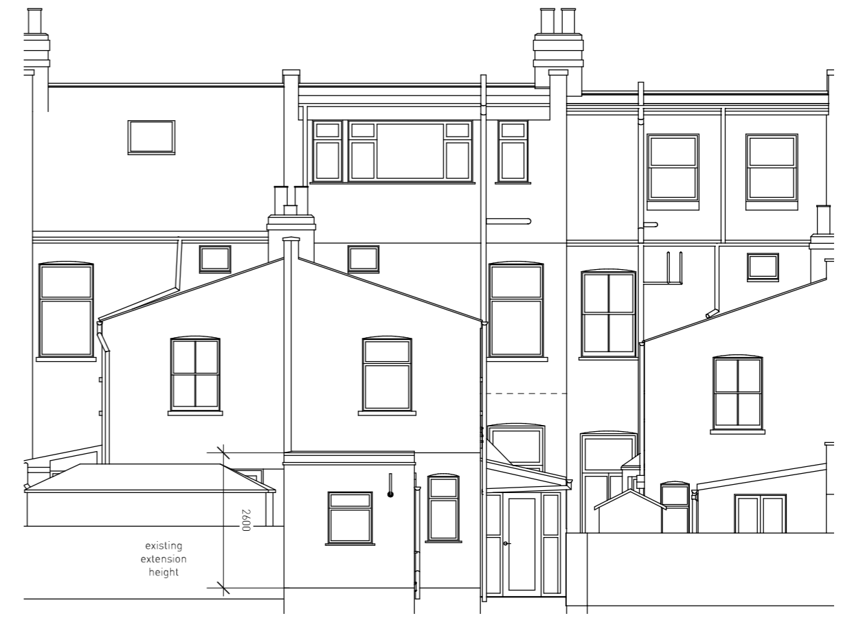
EXISTING REAR ELEVATION 1:200
