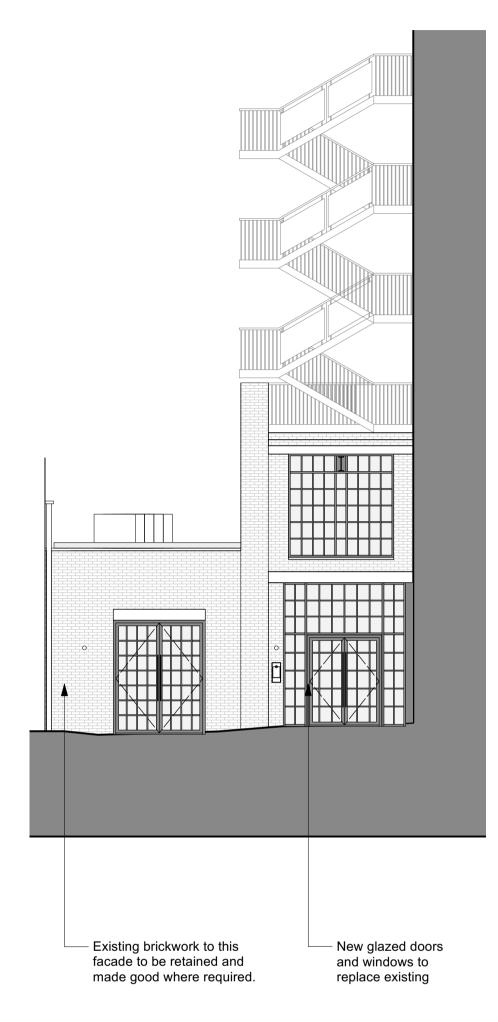
Proposed elevation - North Scale: 1:100
