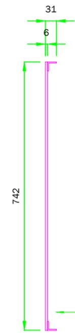
○ **Base Plate: End Elevation**
