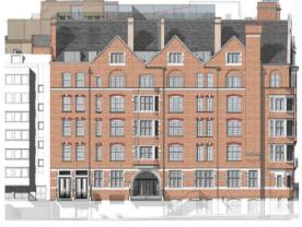
Replacement of existing poor quality window units (from 1990s) to improve thermal efficiency in a drive toward net-zero carbon emissions in operation. The new windows will better reflect the historic window designs. Coupled with improvements to all entrances.
