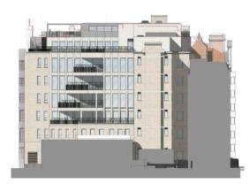
Replacement of the building's mechanical and electrical systems to provide an all electric building that is carbon net-zero in operation. Locating external mechanical systems to the east and south, away from neighbours.
