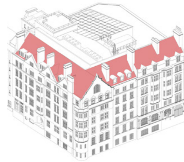
2 1990's development by TP Bennett - Replacement of original slate roofs
