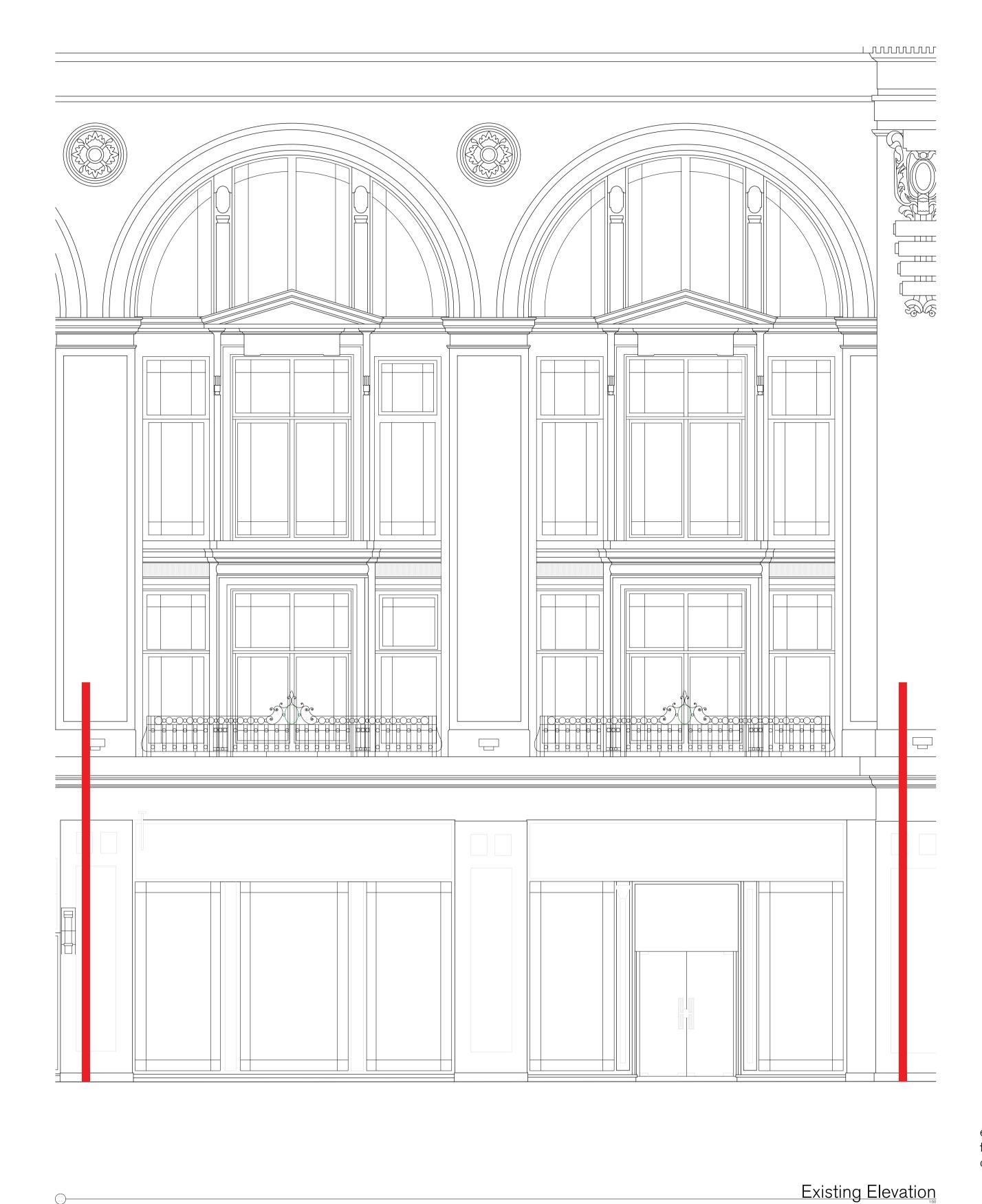
Existing frameless glass doors to be — replaced by framed glass doors within New Reveal to be formed to match adjacent entrance details, existing glazing to be carefully removed and new entrance to be formed within existing shop front. New framed doors and glazed overpanel to be installed, finish of doors to be PPC aluminium in existing entrance. Finish of doors to be PPC aluminium in Bronze / Brown to Bronze / Brown to match existing. match existing. Proposed Elevation
