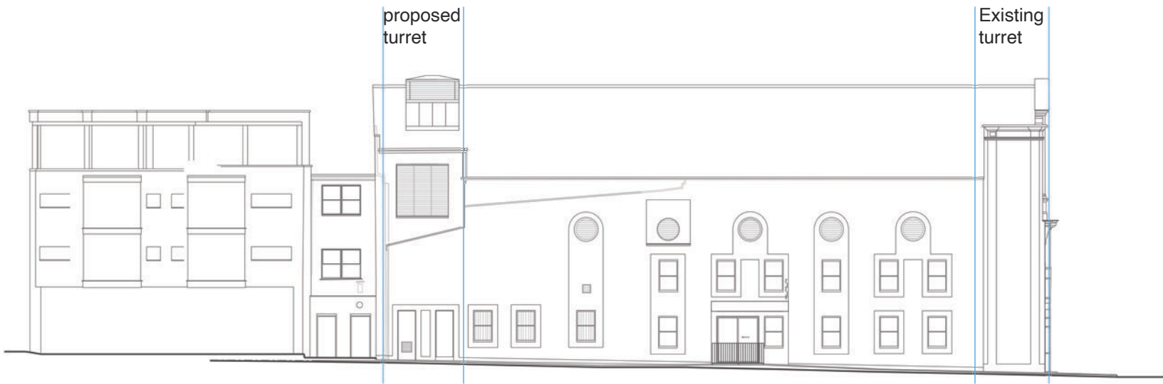
Proposed Grafton Yard elevation viewed from Prince of Wales Road, showing proposed new ventilation turret and plant access opening (canopy and front elevation as planning approved scheme)
