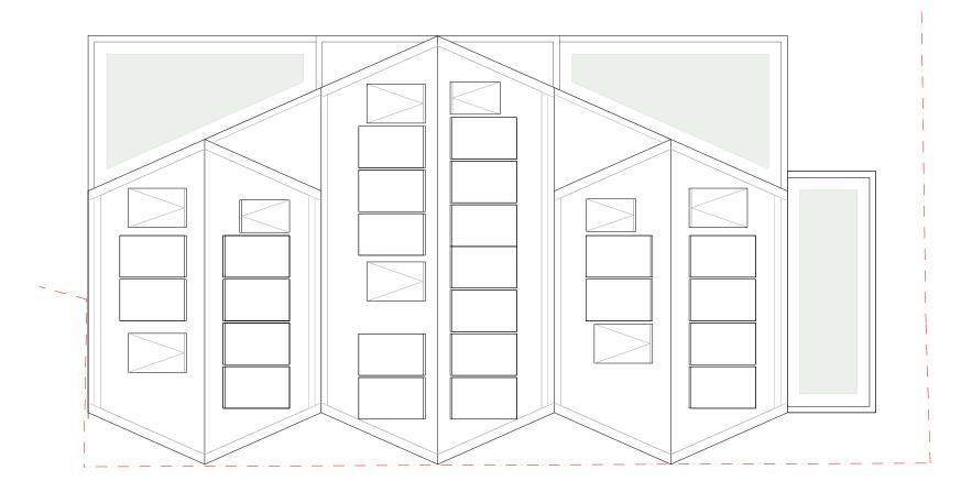
Although the original planning drawings showed green roofs on all flat roofs, having liaised with Sky Garden, it is only possible to have green roofs on the larger elements. This is because a 300mm Riverstone border is required around the area of green roof and therefore on the smaller roofs, this would become a ballast only roof.
