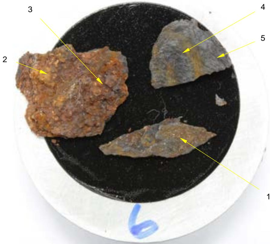
Figure 13: Paint from Area 1 examined using EDX analysis, showing analysis positions.
