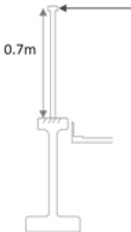
Figure B Idealised structure for parapet
