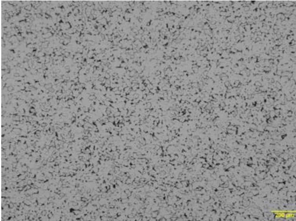
Figure 15: Etched RM micrograph showing typical carbon steel microstructure.
