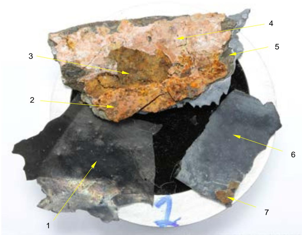
Figure 17: Paint from Area 2 examined using EDX analysis, showing analysis positions.
