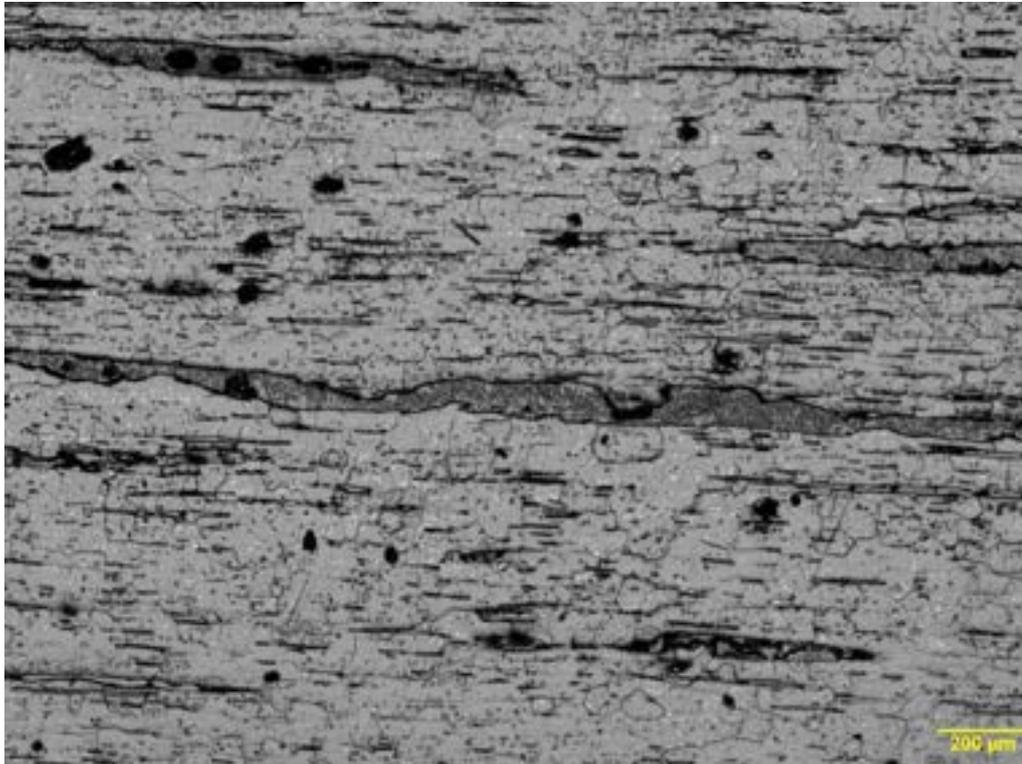
Figure 11: Etched RM micrograph showing typical wrought iron microstructure.
