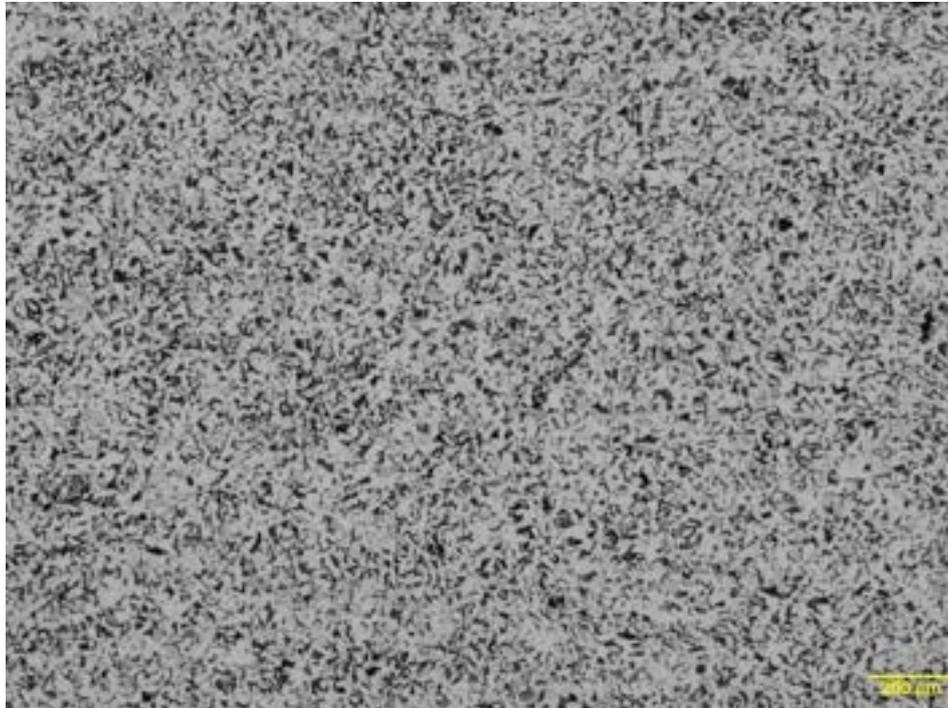
Figure 19: Etched RM micrograph showing typical carbon steel microstructure.
