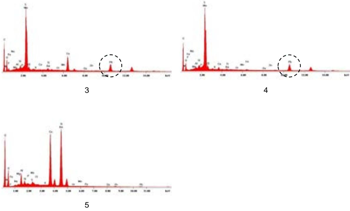
Figure 31: EDX spectra of numbered analysis positions from paint sample.
