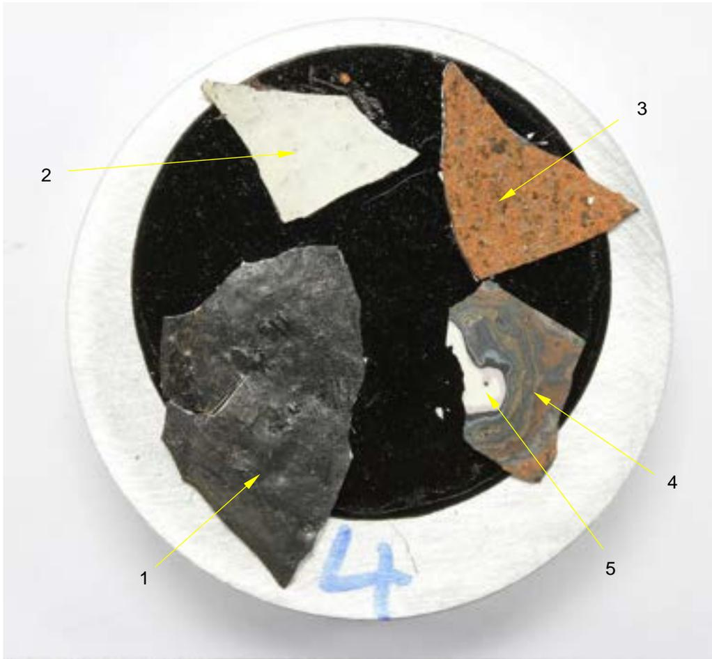
Figure 30: Paint from Area 5 examined using EDX analysis, showing analysis positions.
