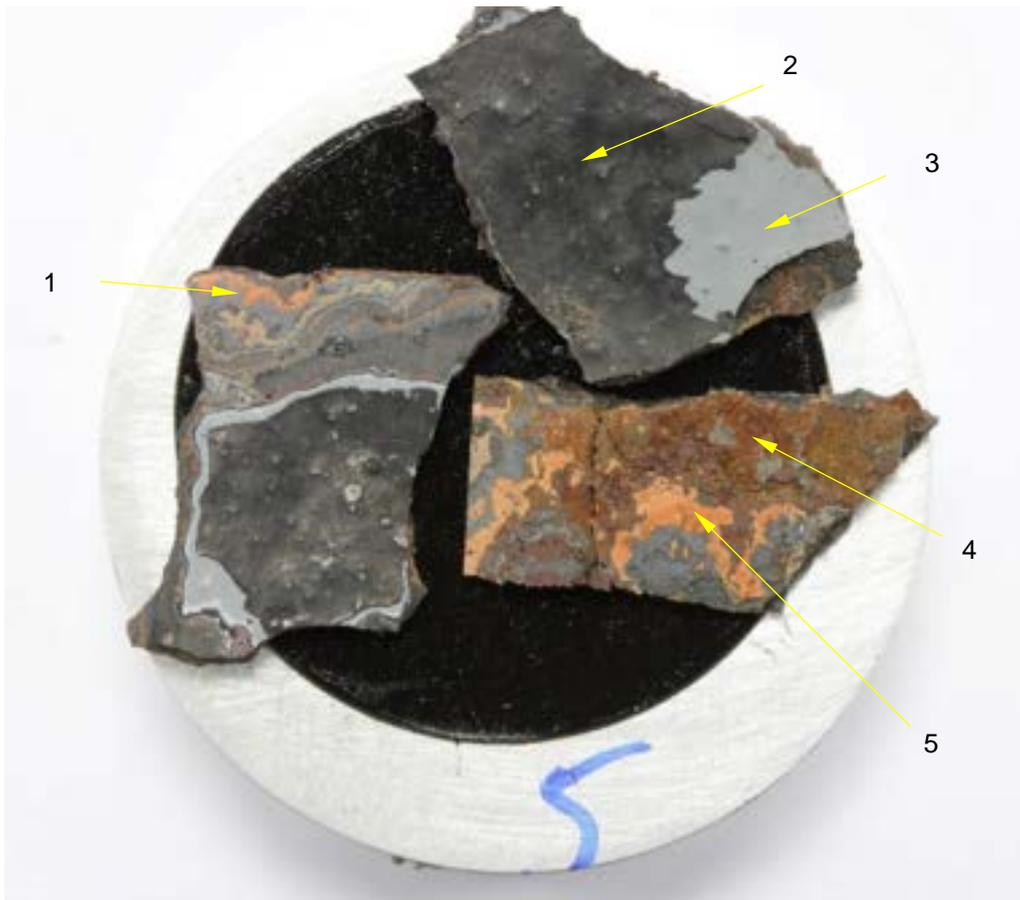
Figure 35: Paint from Area 6 examined using EDX analysis, showing analysis positions.
