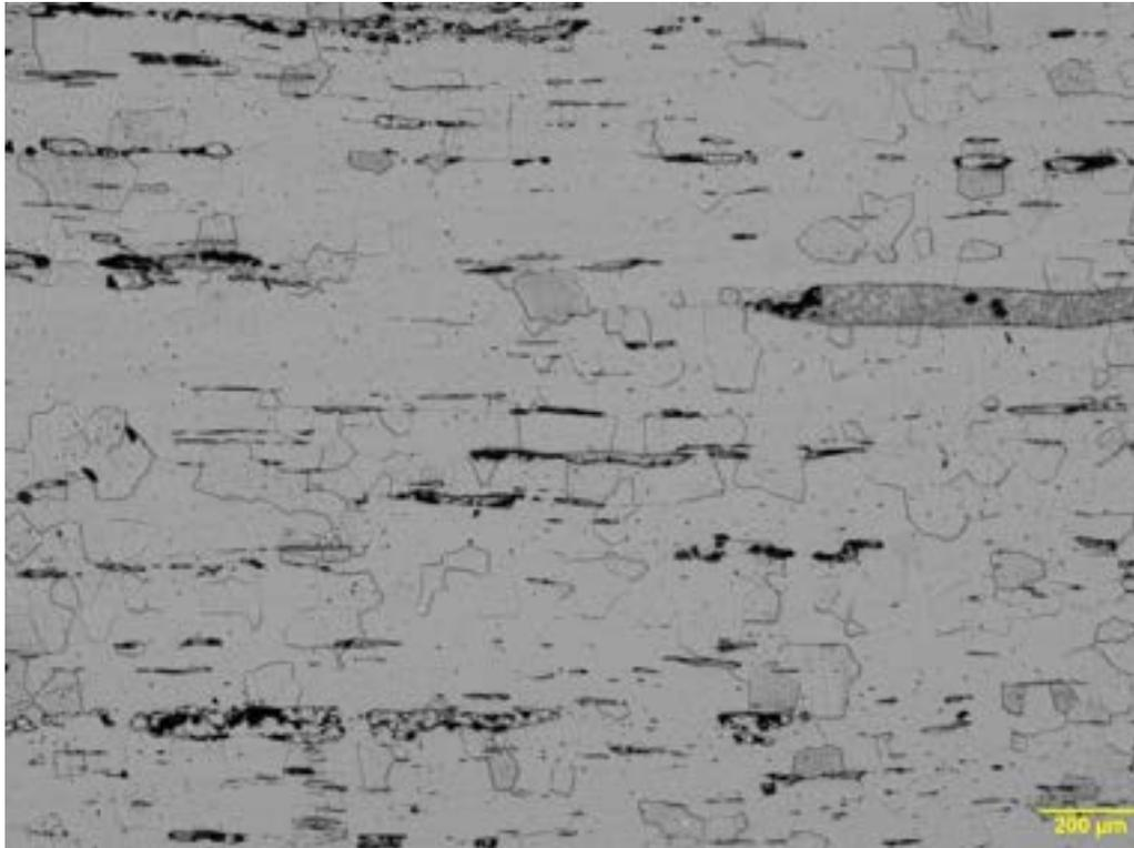
Figure 24: Etched RM micrograph showing typical wrought iron microstructure.
