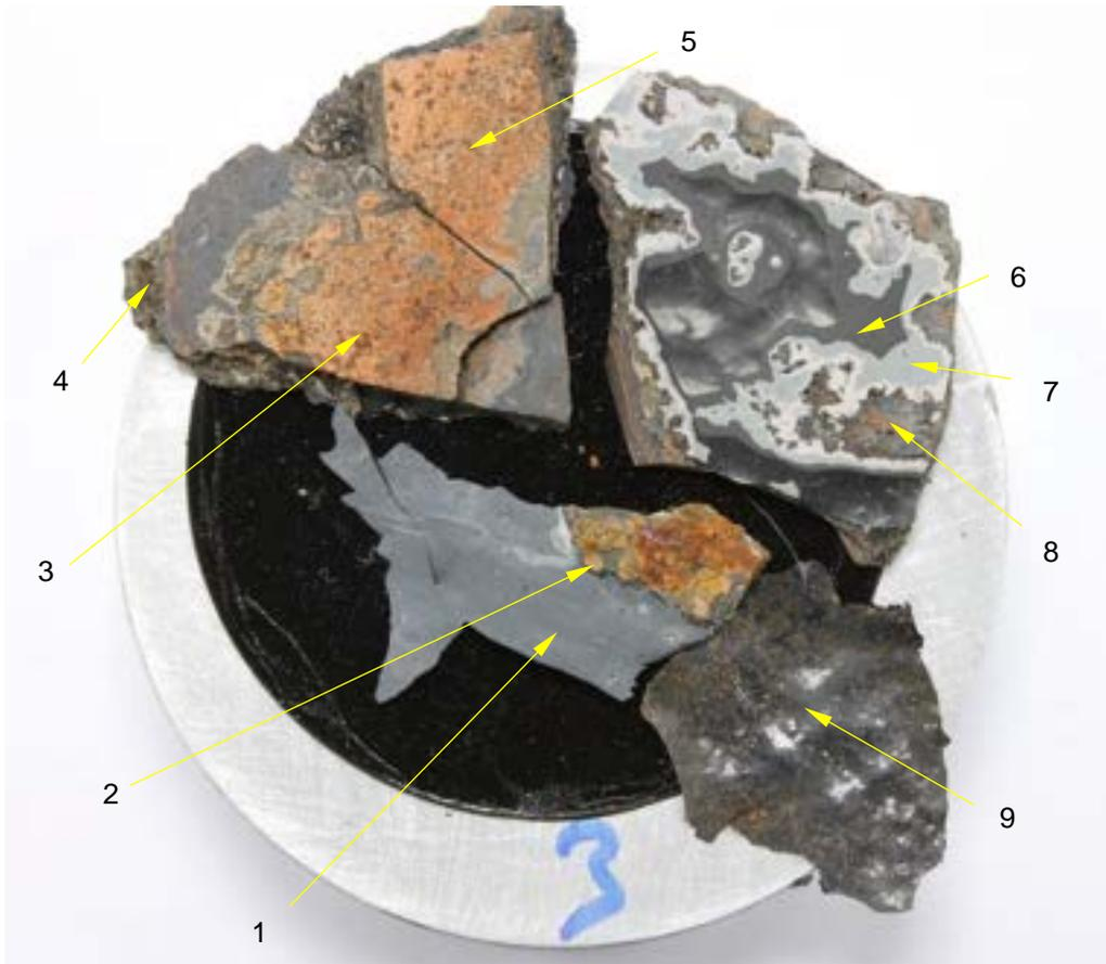
Figure 26: Paint from Area 4 examined using EDX analysis, showing analysis positions.
