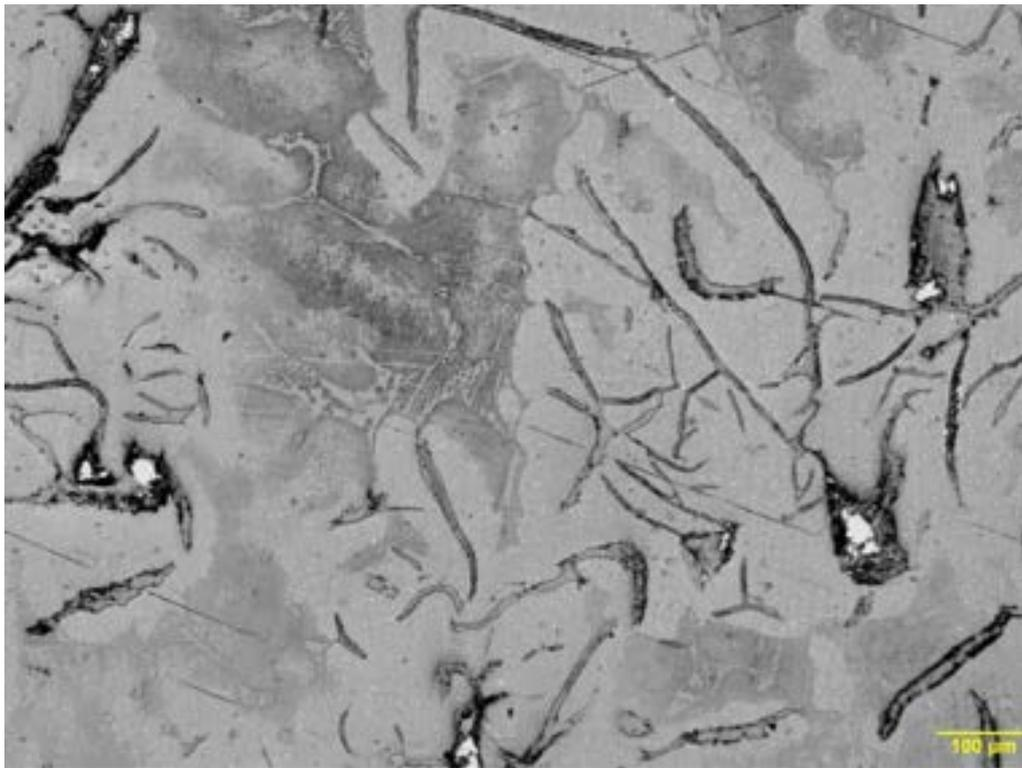
Figure 33: Etched RM micrograph showing typical grey flake cast iron microstructure.
