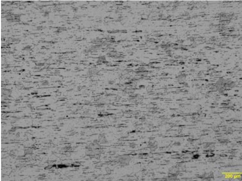
Figure 28: Etched RM micrograph showing typical wrought iron microstructure.
