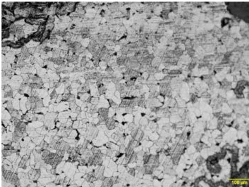
Figure 20: Etched micrograph of sample removed from structure, showing typical carbon steel microstructure.
