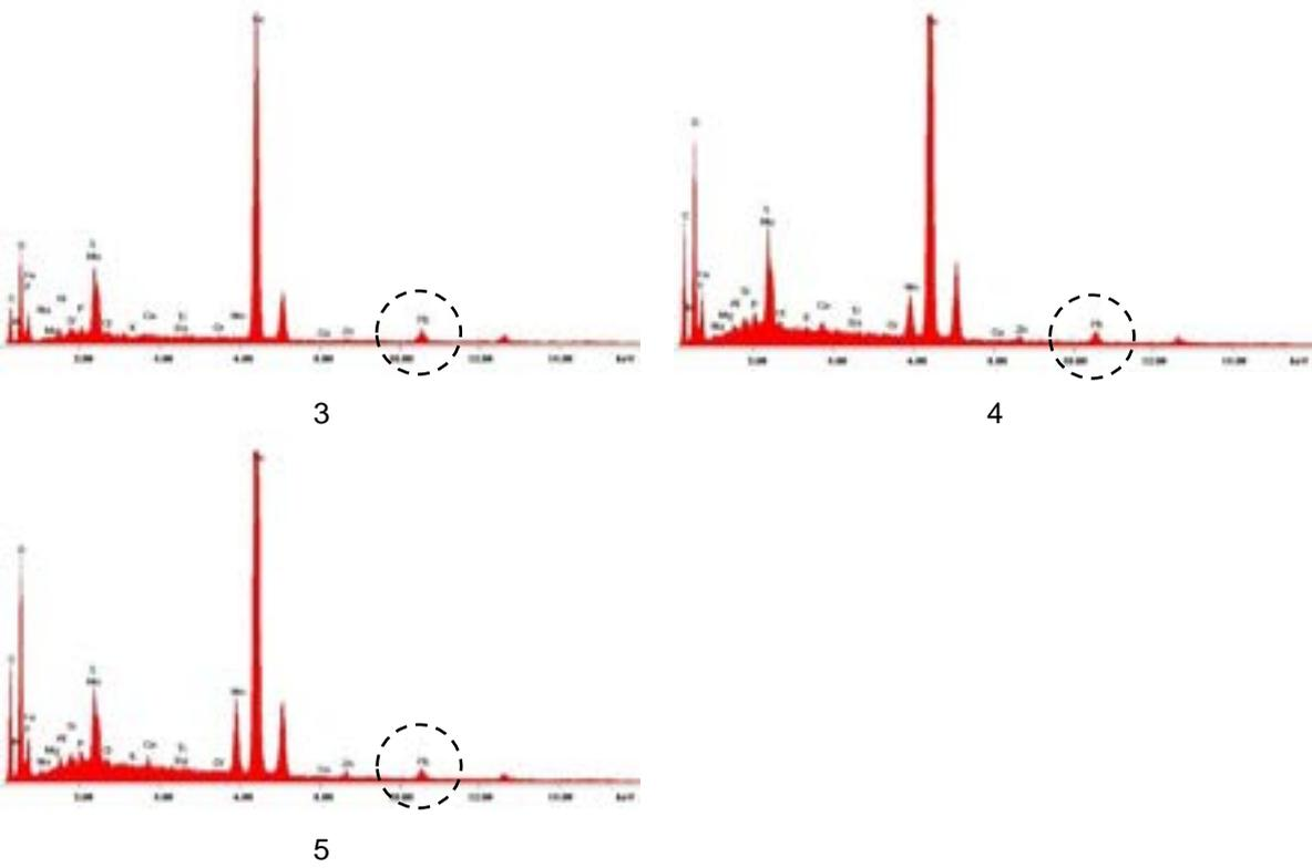
Figure 14: EDX spectra of numbered analysis positions from paint sample.
