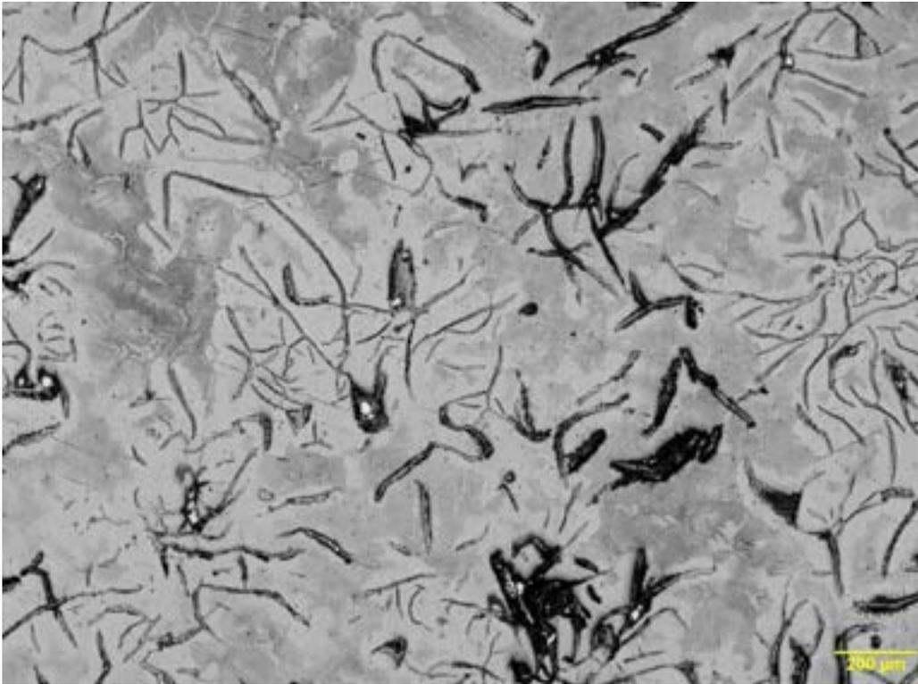
Figure 32: Etched RM micrograph showing typical grey flake cast iron microstructure.
