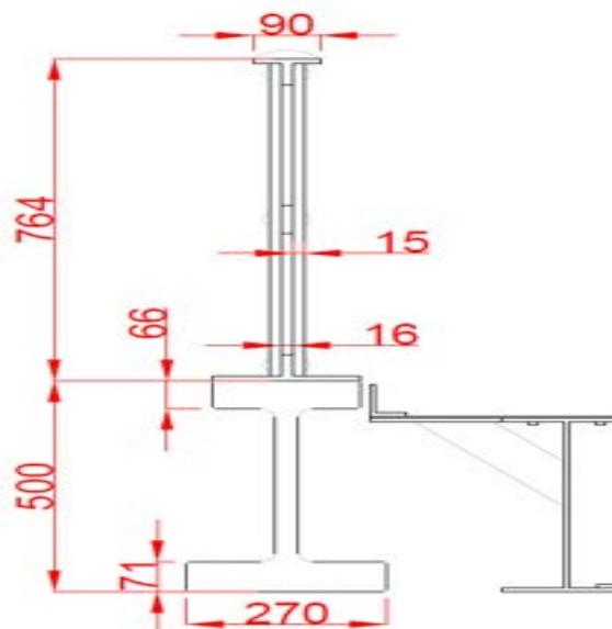
**Cross section of the parapet**
