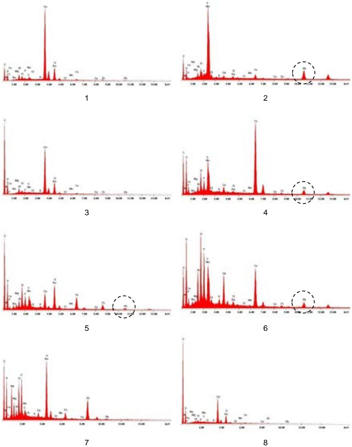
Figure 23: EDX spectra of numbered analysis positions from paint sample.
