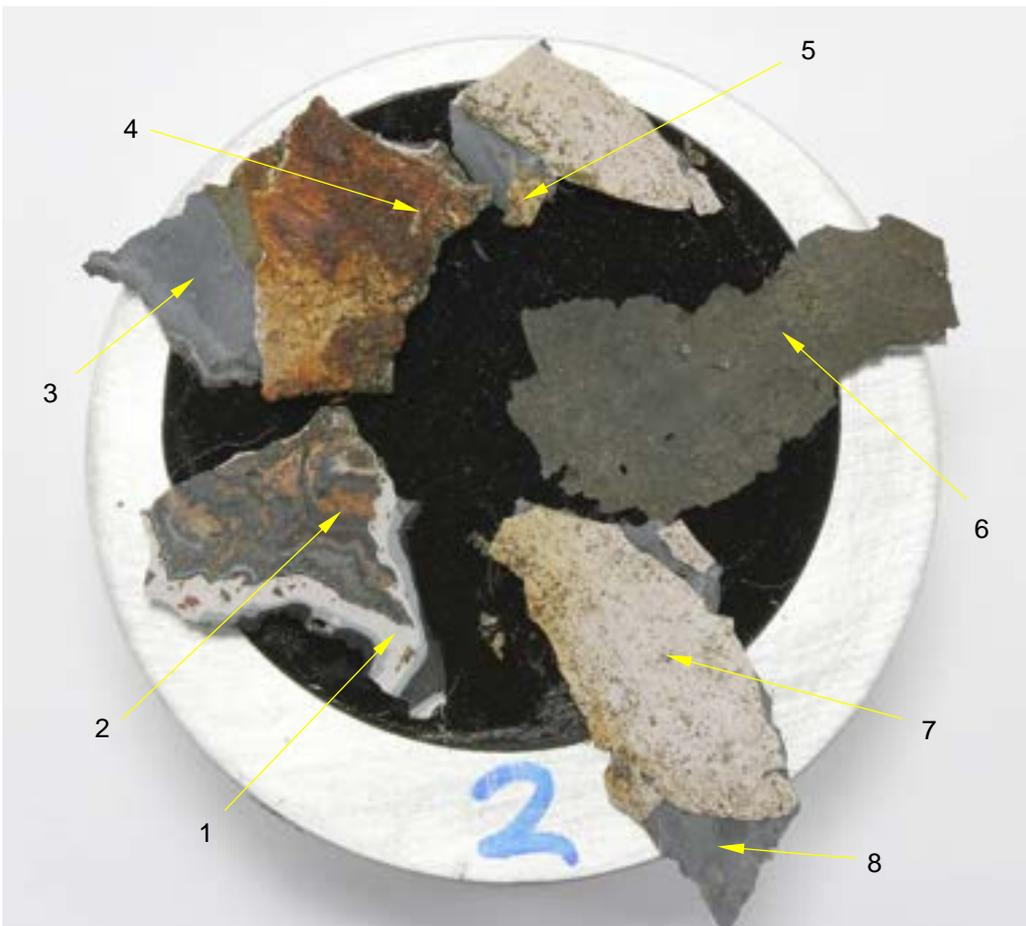
Figure 22: Paint from Area 3 examined using EDX analysis, showing analysis positions.
