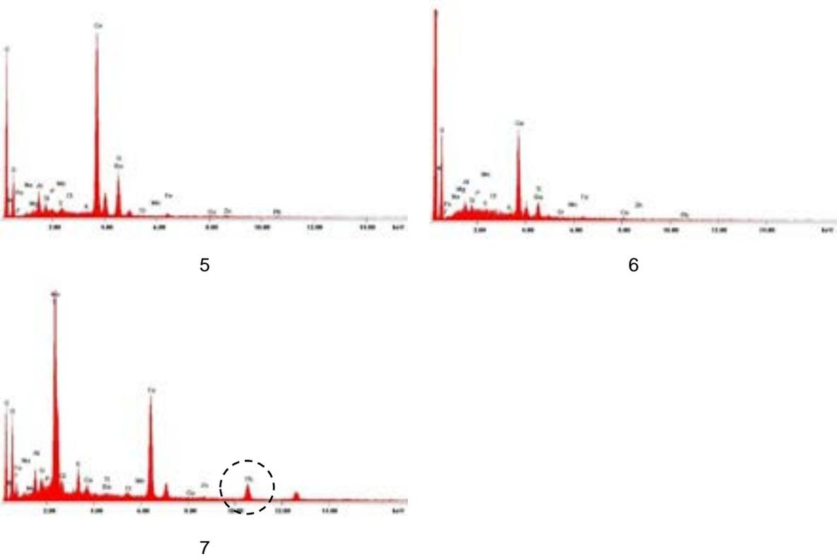
Figure 18: EDX spectra of numbered analysis positions from paint sample.
