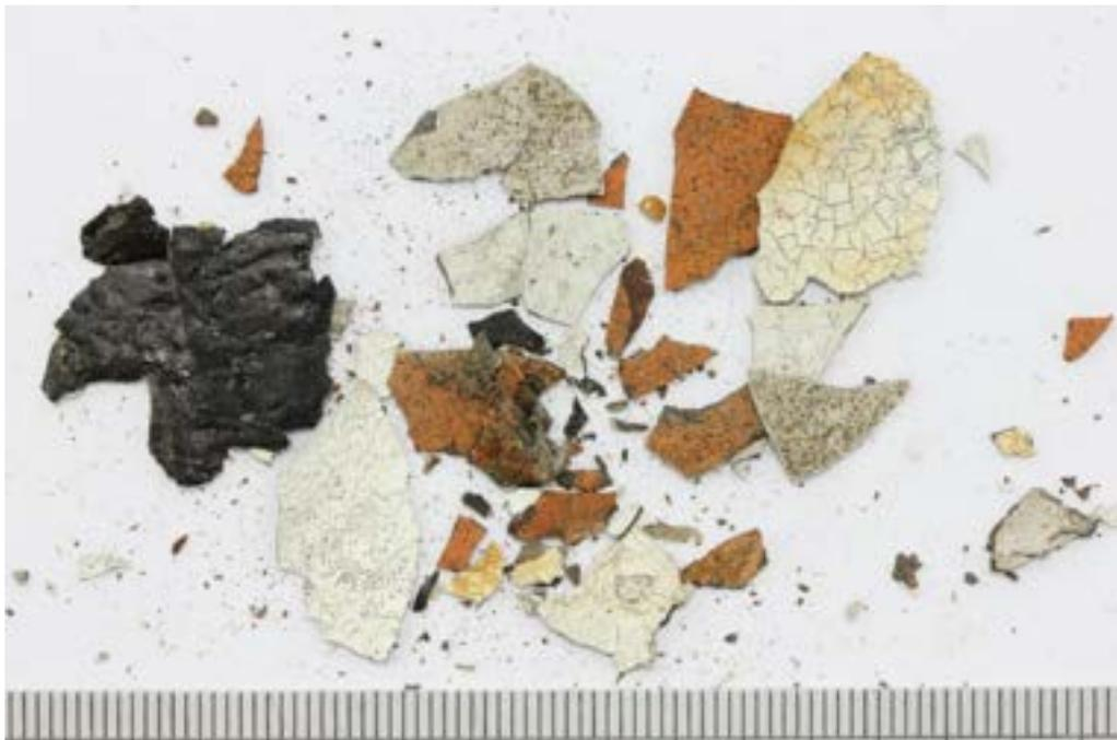
Figure 29: Paint sample collected from Area 5.
