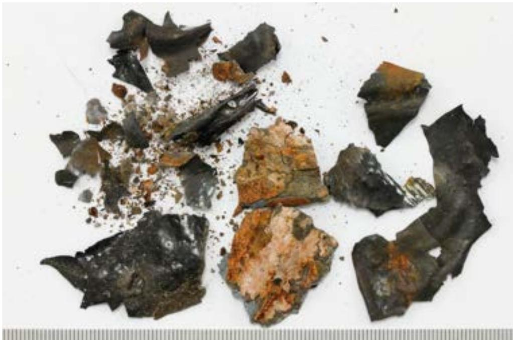
Figure 16: Paint sample collected from Area 2.
