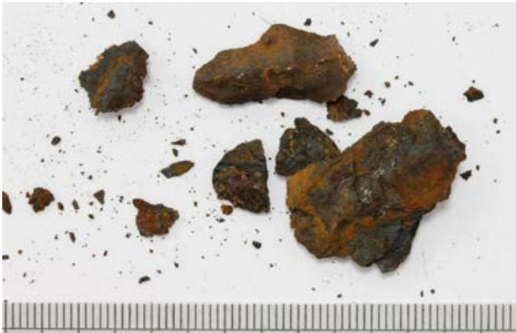
Figure 12: Paint sample collected from Area 1.
