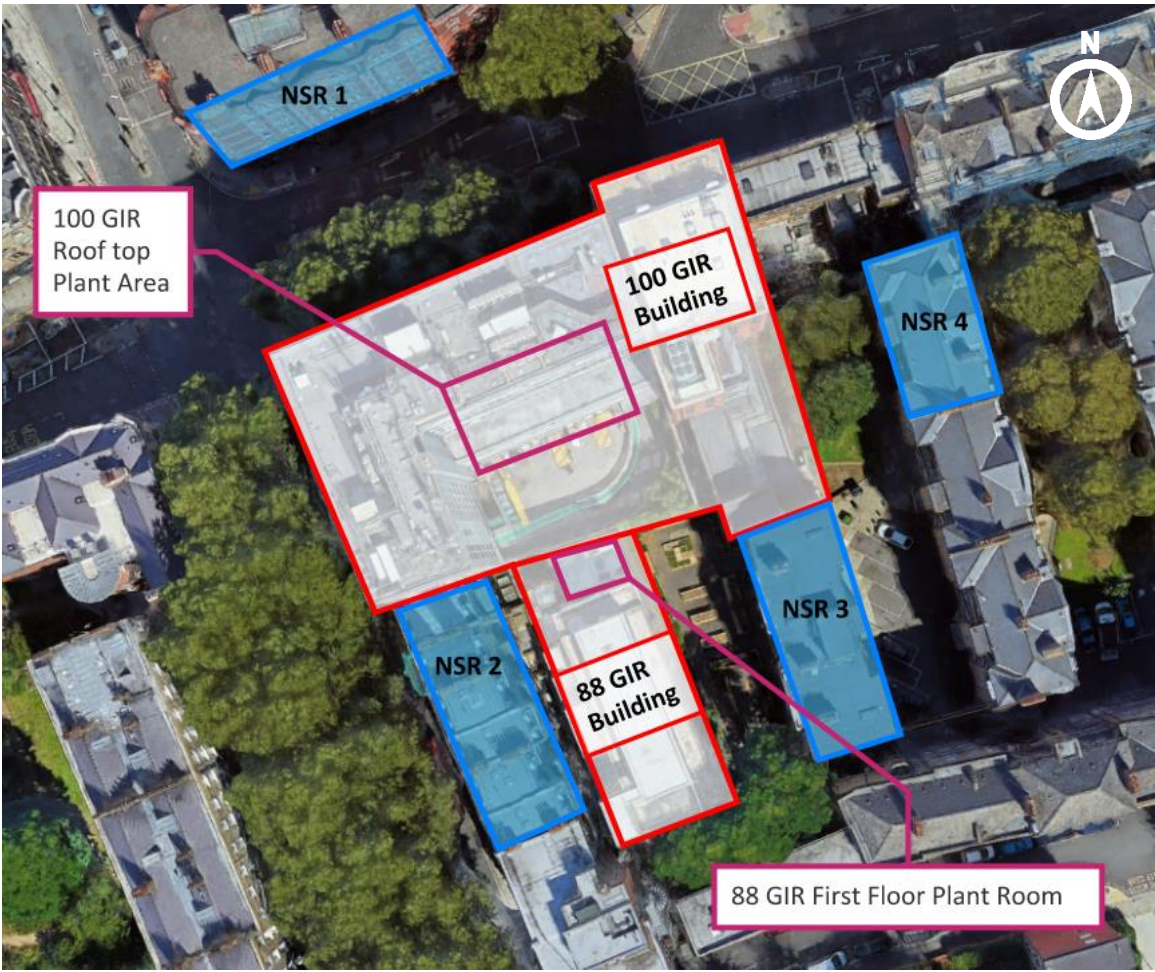
Figure 11 - Aerial image site showing location of external plant and noise sensitive receivers (NSRs).
