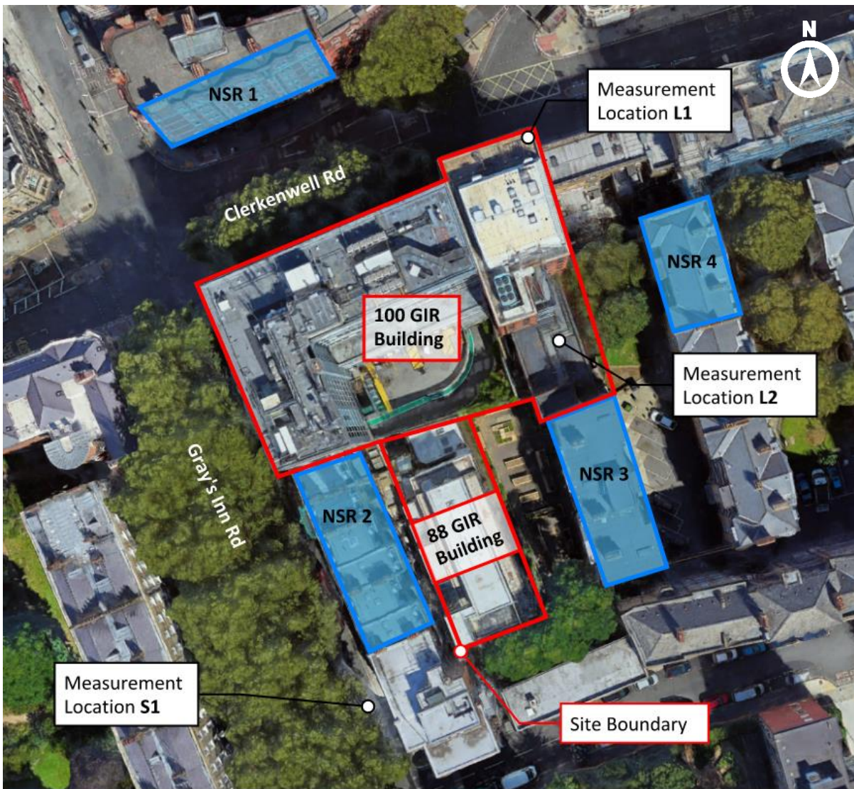
Figure 5 - Aerial image site showing proposed development, noise sensitive receivers (NSRs), and measurement locations (L1 & L2).
