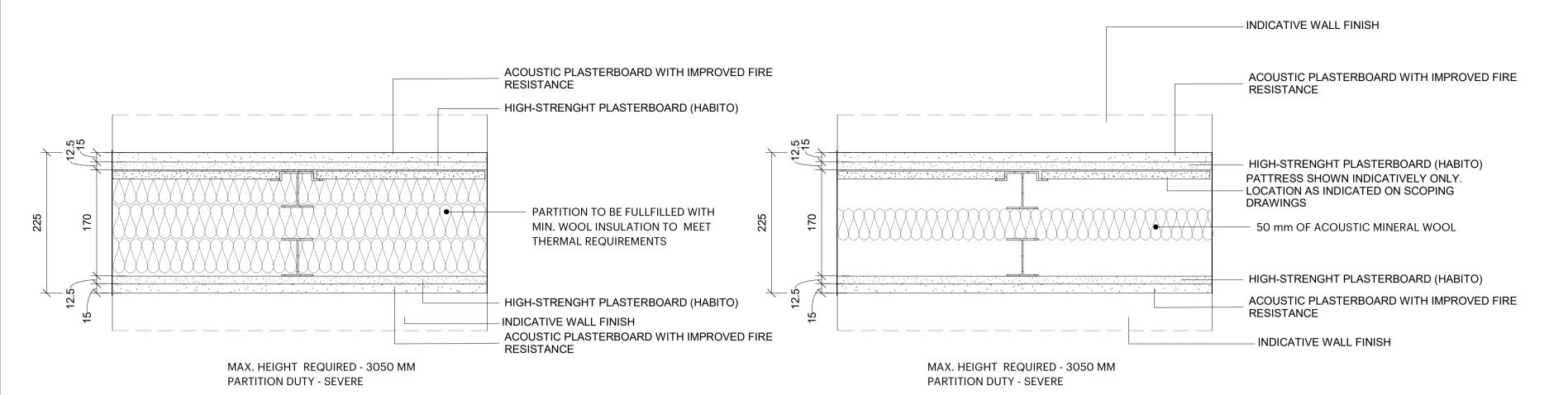
THERMAL - 0.19 W/m2K FIRE RATING 120/120 ACOUSTIC RATING 50 DnTw + Ctr
