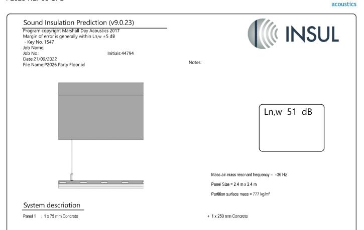
Frame: Suspended Light Steel Grid (2.5E2 mm x 45 mm ), Stud spacing  $\,$  600 mm ; Cavity Width 250 mm Panel 2 - : 2 x 12.5 mm Gyproc Wallboard 12.5mm
