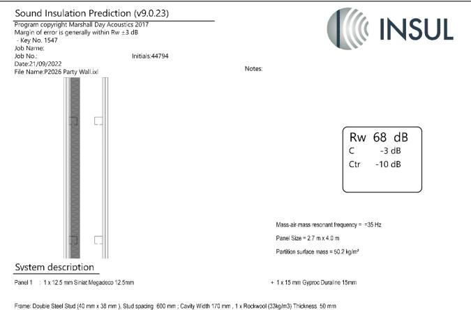
Frame: Double Steel Stud (40 mm x 38 mm ), Stud spacing 600 mm ; Cavity Width 170 mm , 1 x Rockwool (33kg/m3) Thickness 50 mm Panel 2 : 1 x 15 mm Gyproc SoundBloc 15mm + 1 x 12.5 mm Siniat Megadeco 12.5mm
