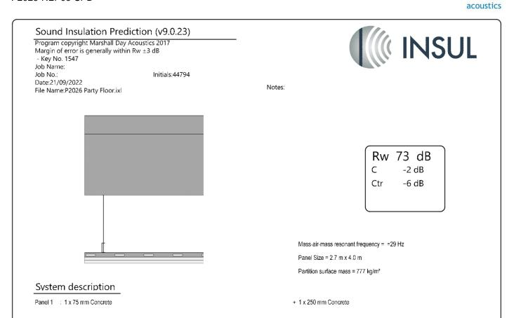
Frame: Suspended Light Steel Grid (2.5E2 mm x 45 mm ), Stud spacing  $\,$  600 mm ; Cavity Width 250 mm Panel 2 - : 2 x 12.5 mm Gyproc Wallboard 12.5mm
