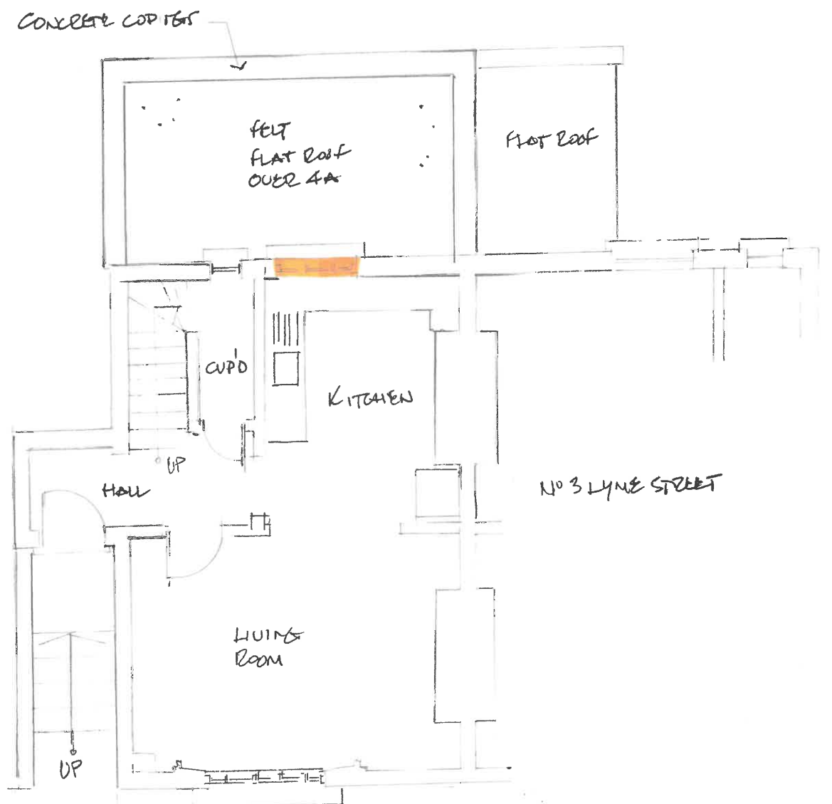
EXISTING GROUND FLOOR SHOWING DEMOLITION AREA
