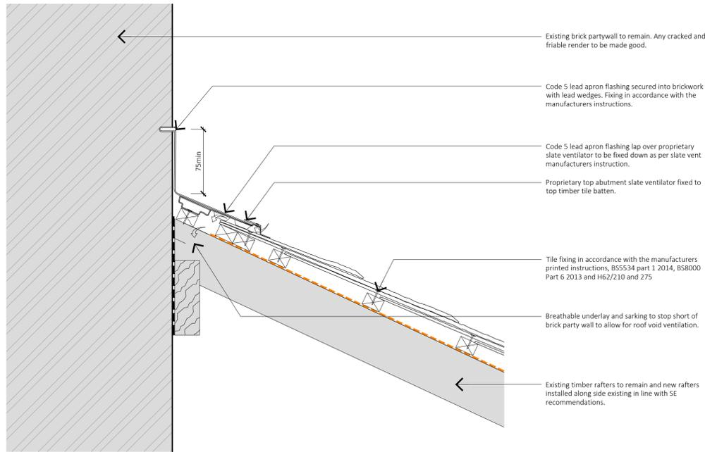
01 DETAIL - MONOPITCH ROOF TOP ABUTMENT
