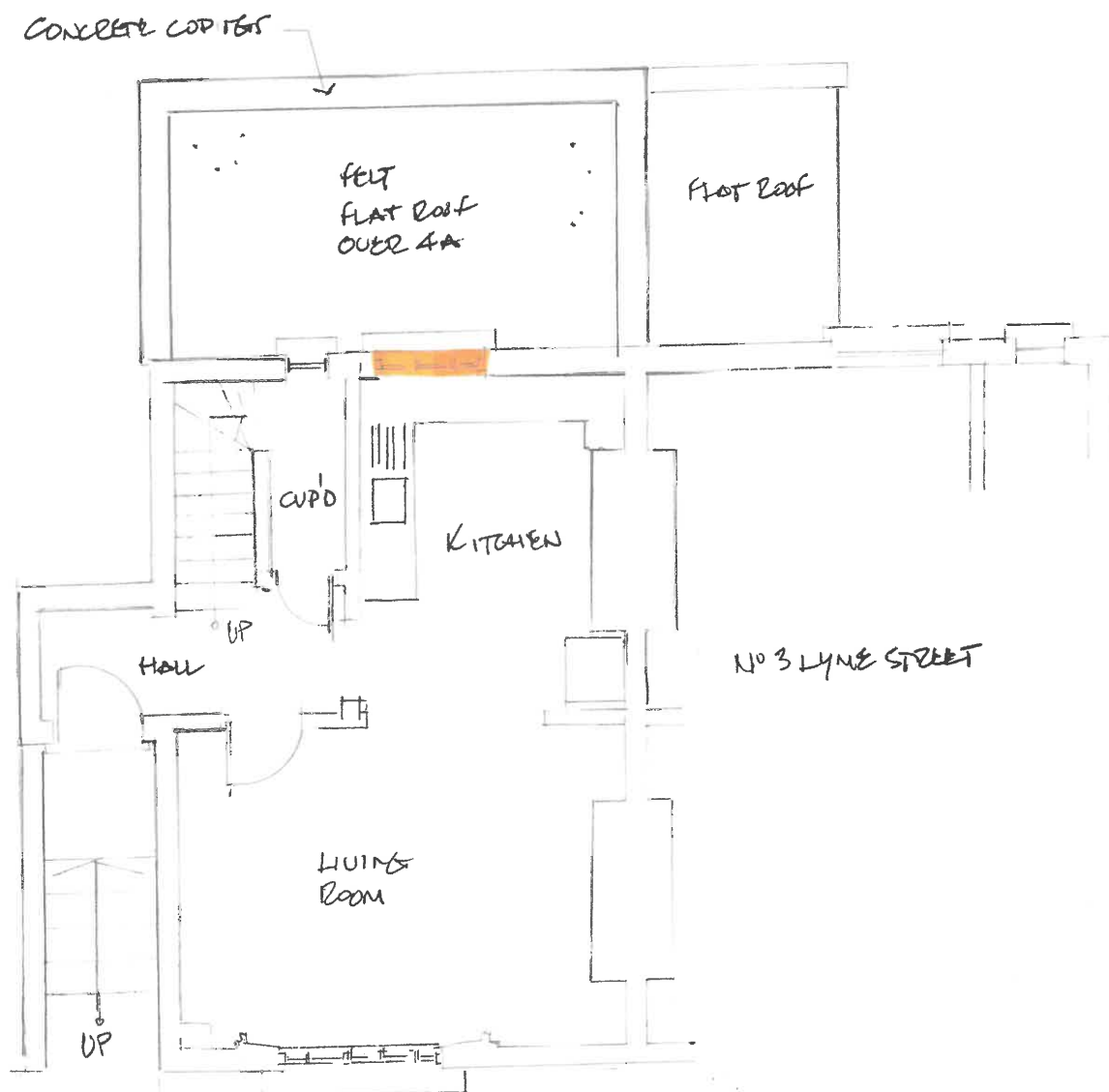
EXISTING GROUND FLOOR SHOWING DEMOLITION AREA
