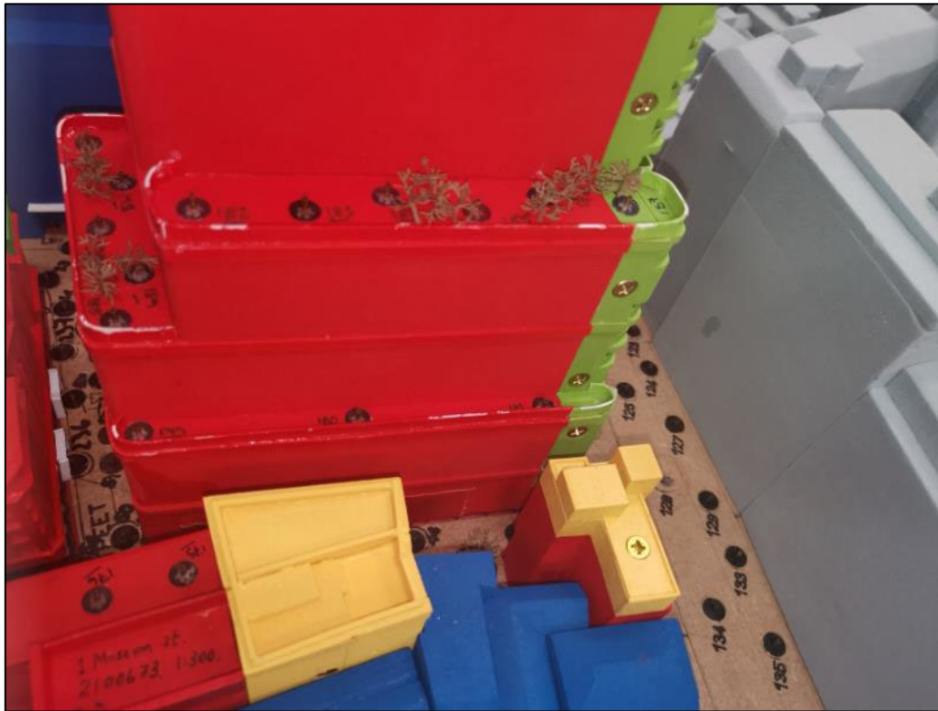
Figure 16: Image of the wind tunnel model showing trees on the upper level terraces; the height of the perimeter balustrade was modelled at 1.4m on all terraces
