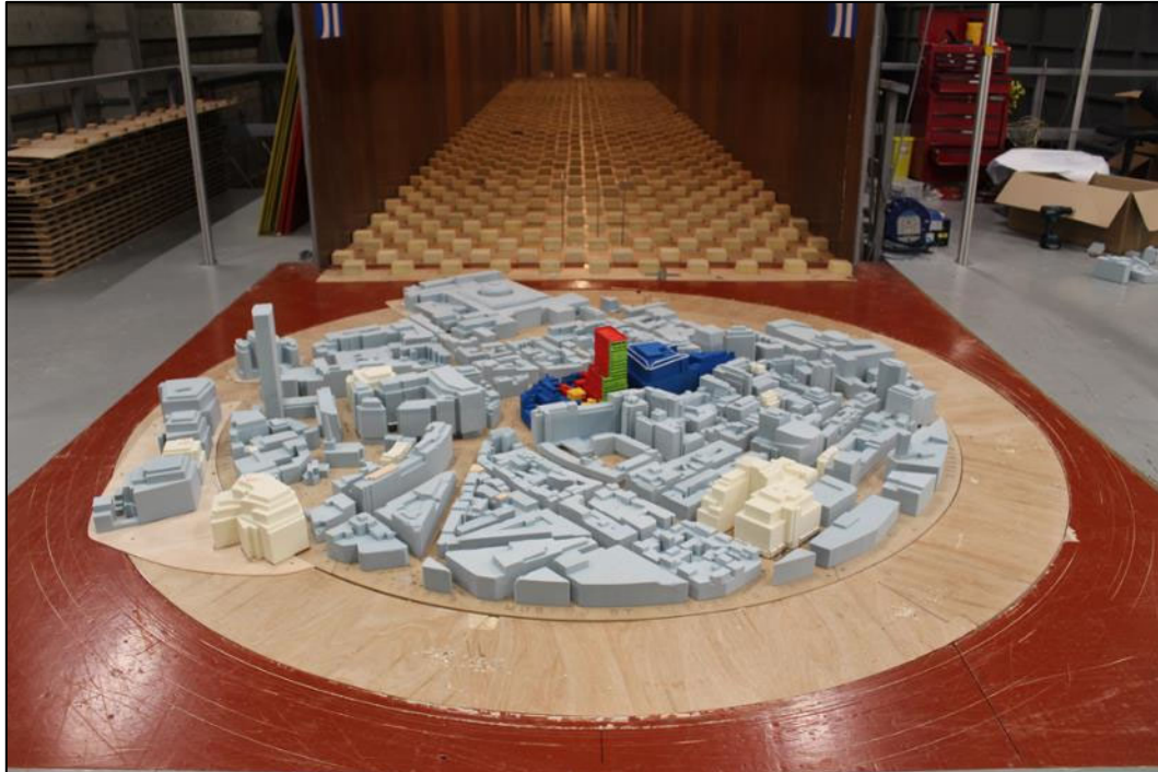
Figure 1: 1:300 scale wind tunnel model including the Proposed Development and cumulative surroundings (view from south)
