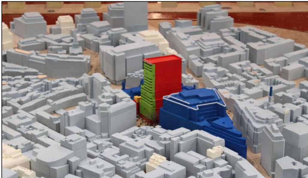
Figure 26: Wind tunnel model of the Proposed Development with Cumulative Surroundings indicated by cream-coloured buildings (view from the East)
