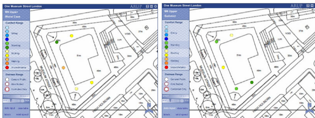
Figure 24: ‘Worst’ and summer season conditions on the roof terrace of the Post Building in presence of the Proposed Development in existing surroundings
