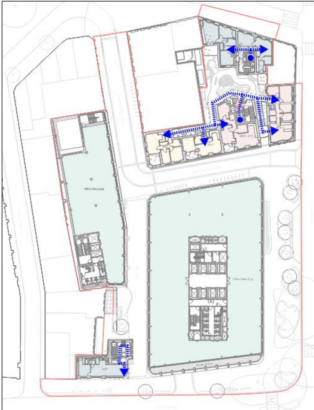
Figure 7 West Central Street & High Holborn upper floor goods distribution routes from on-street loading locations
