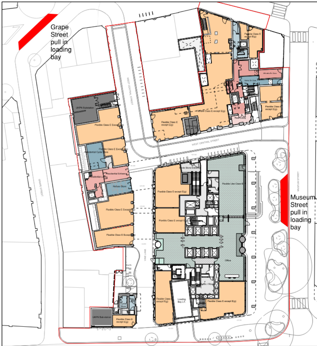
Figure 5 Ground floor loading bays
