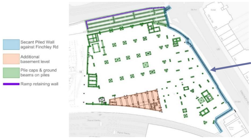
Figure 3 Existing O2 Basement Structure
