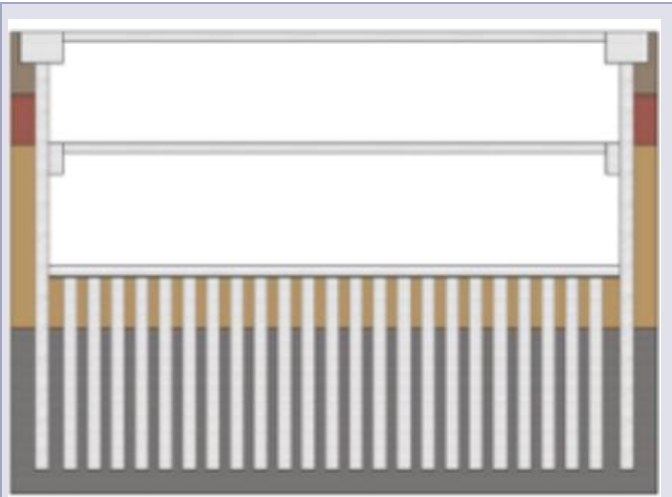
6- Install base slab followed by intermediate floor followed by removal of intermediate temporary prop.
