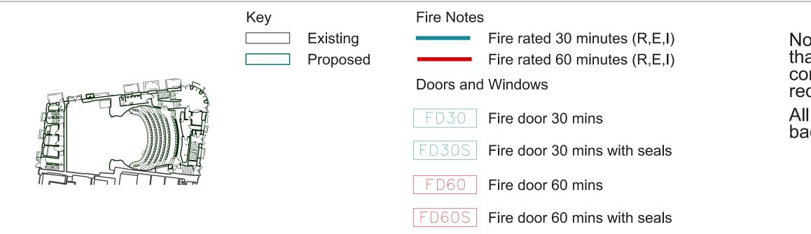
Note: all existing doors along existing fire escapes that are unaffected by the proposed works are considered FD30 doors - no additional works are required to these doors to increase their fire rating All new doors along the new compartment wall at back of stalls to be FD60s
