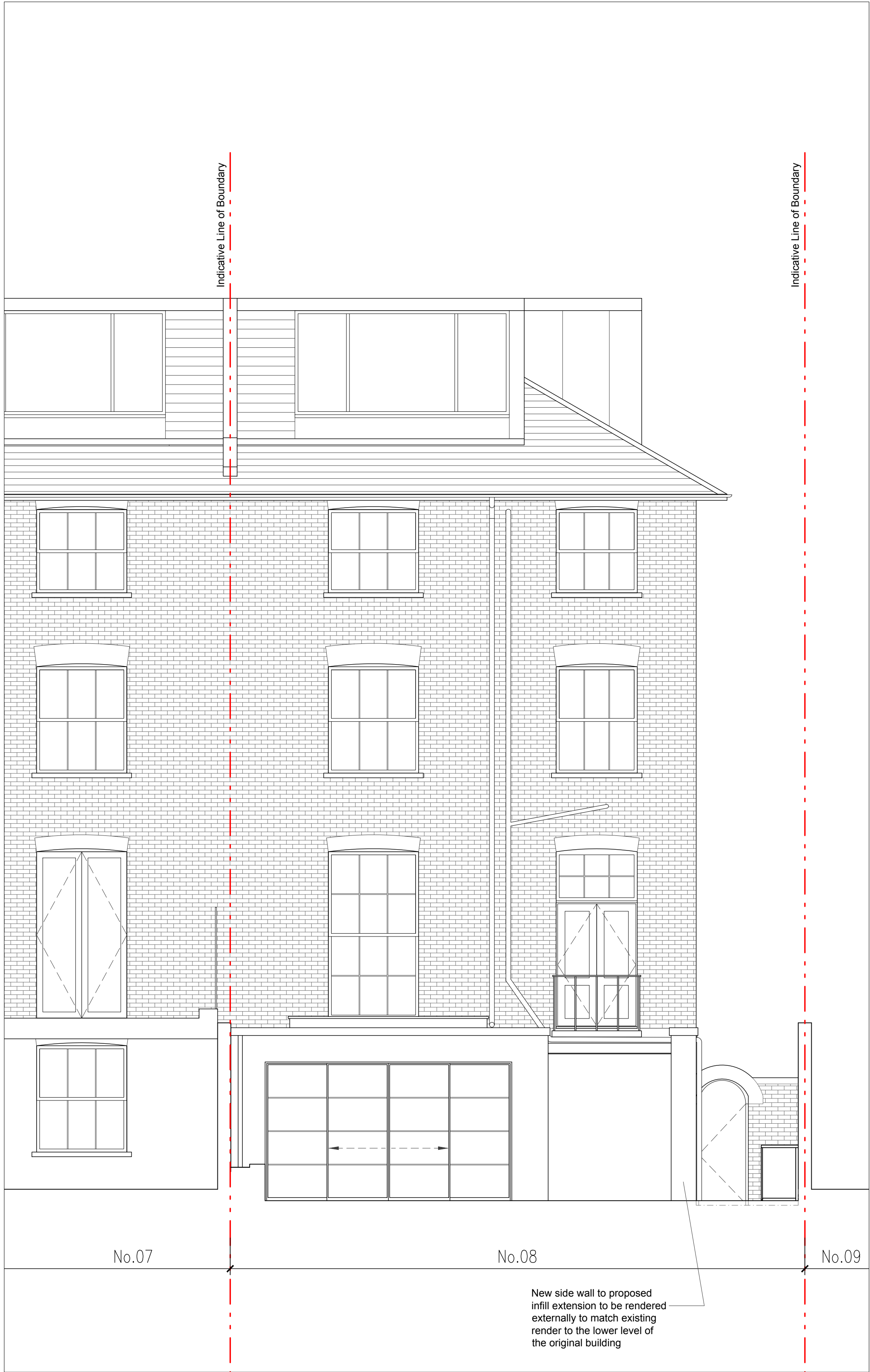
Proposed South East | Rear Elevation Scale 1:100 @ A3 | 1:50 @ A1
