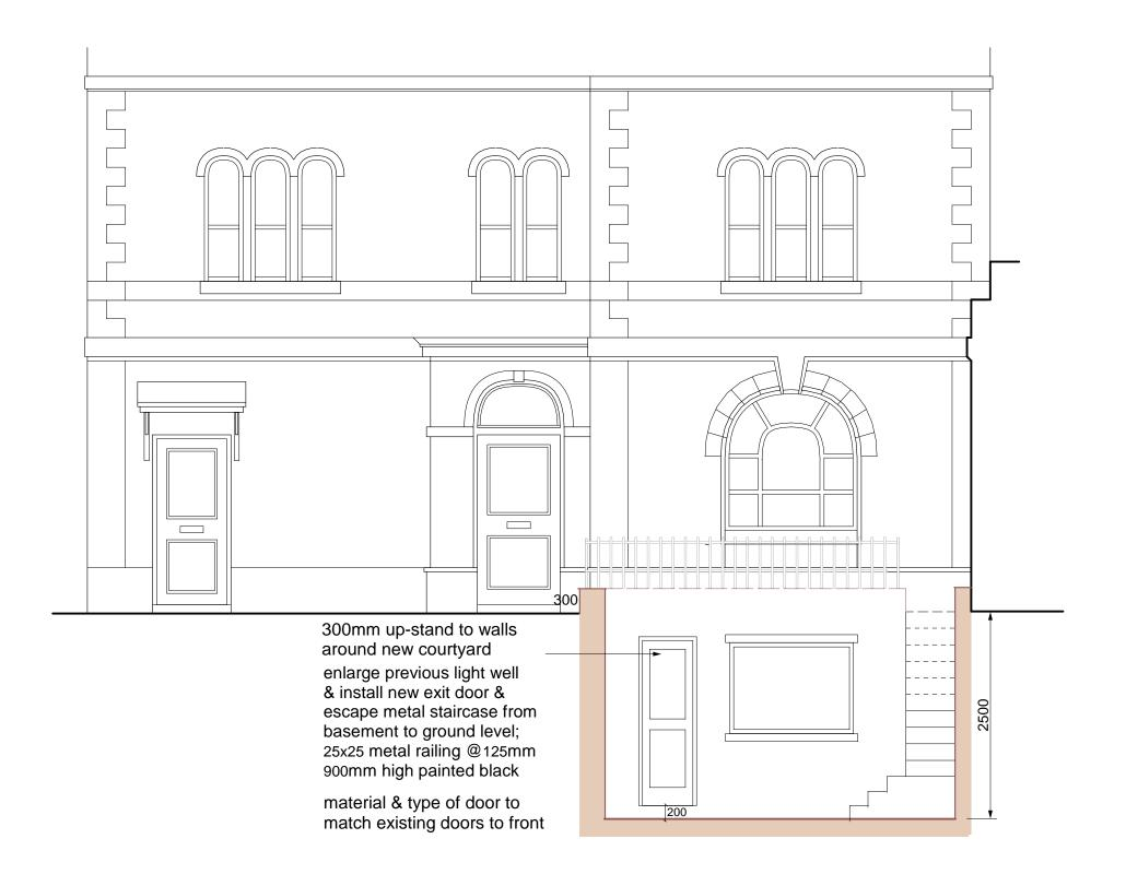
PROPOSED FRONT ELEVATION-SECTION
