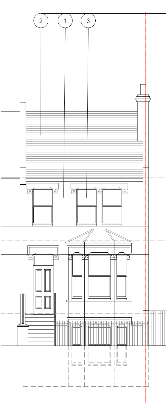
01 Existing Front Elevation Scale:1:100
