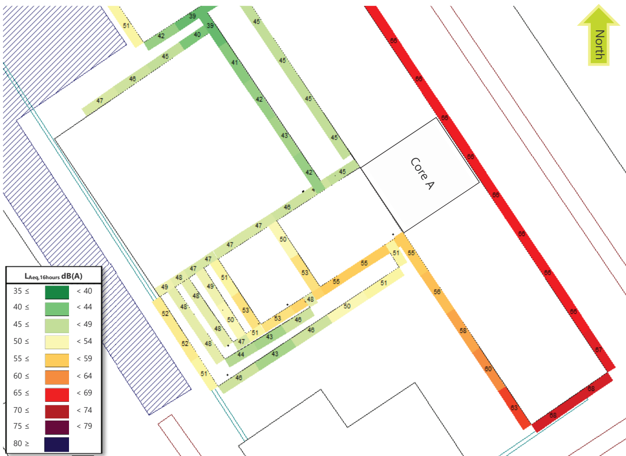
Figure 3-5: Predicted highest daytime Cores A to B, Institute of Education façade incident noise levels (L Aeq,T dB(A))
