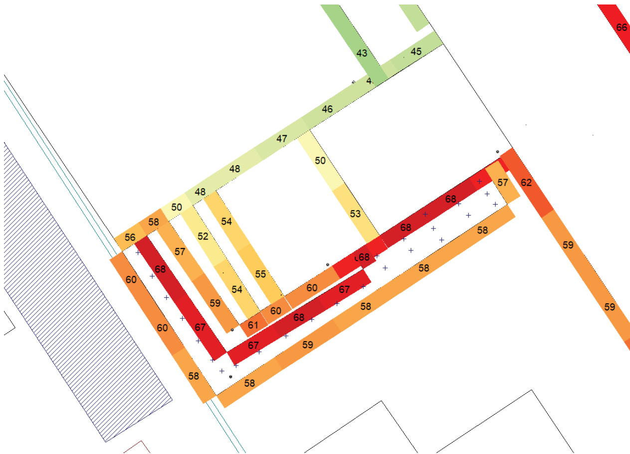
Figure 3-6: Daytime L_{Aeq,T} noise levels with bar terrace at full capacity – south and west elevations
