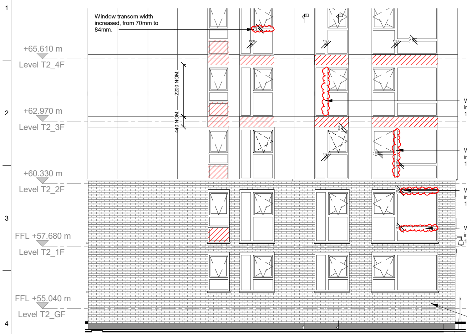
1 Interface with brickwork podium Elevation 1 : 100
