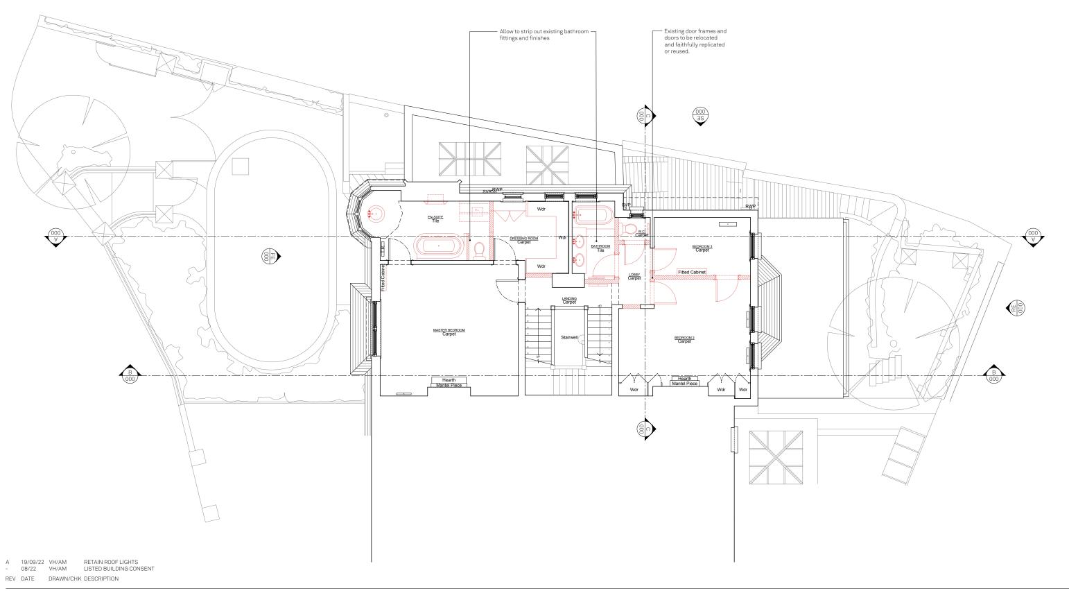
**GAINSBOROUGH GARDENS** GA012 revA EXISTING 2ND FLOOR DEMOLITION PLAN Do not scale for construction. Use figured dimensions only.
