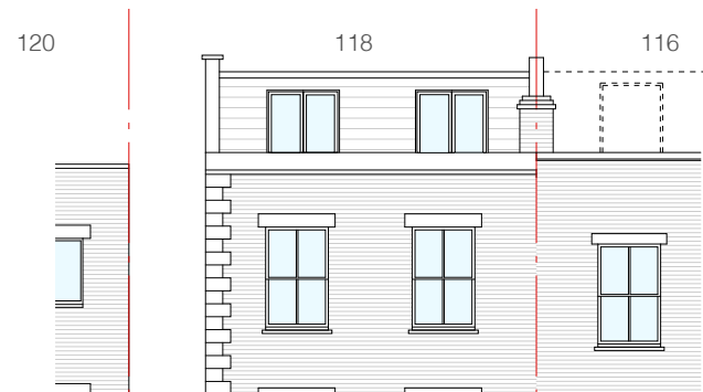
front elevation of proposed mansard extension
