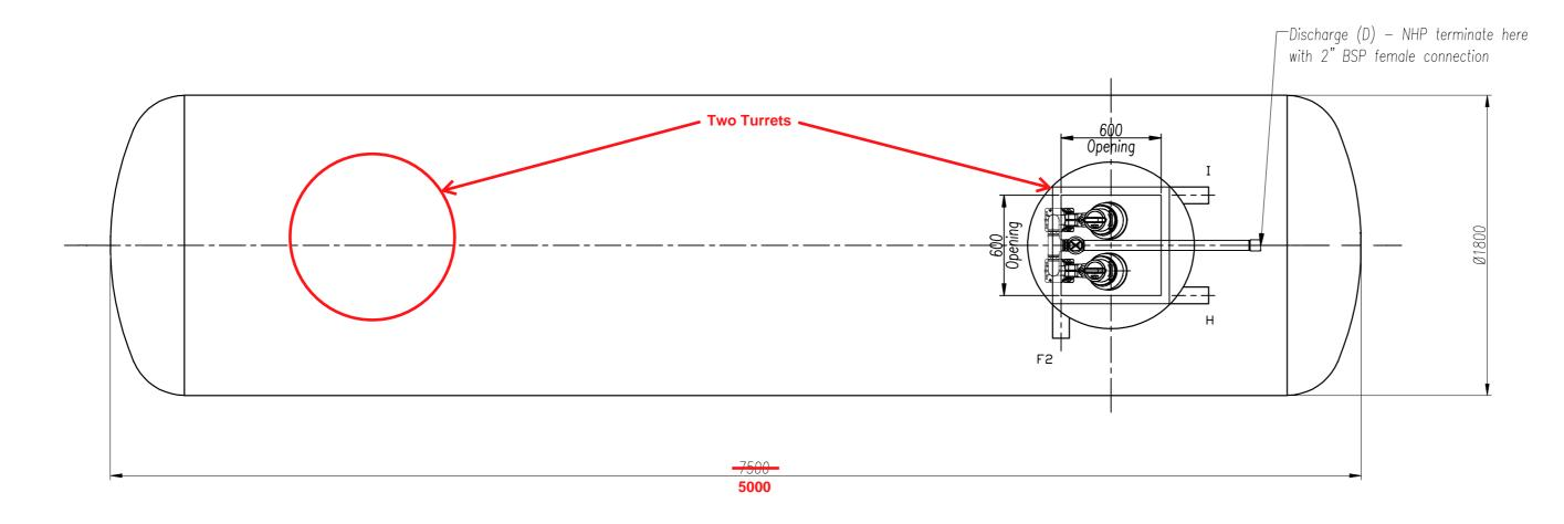
Tank manufactured to tolerance of  $\pm 10$ mm on all dimensions.
