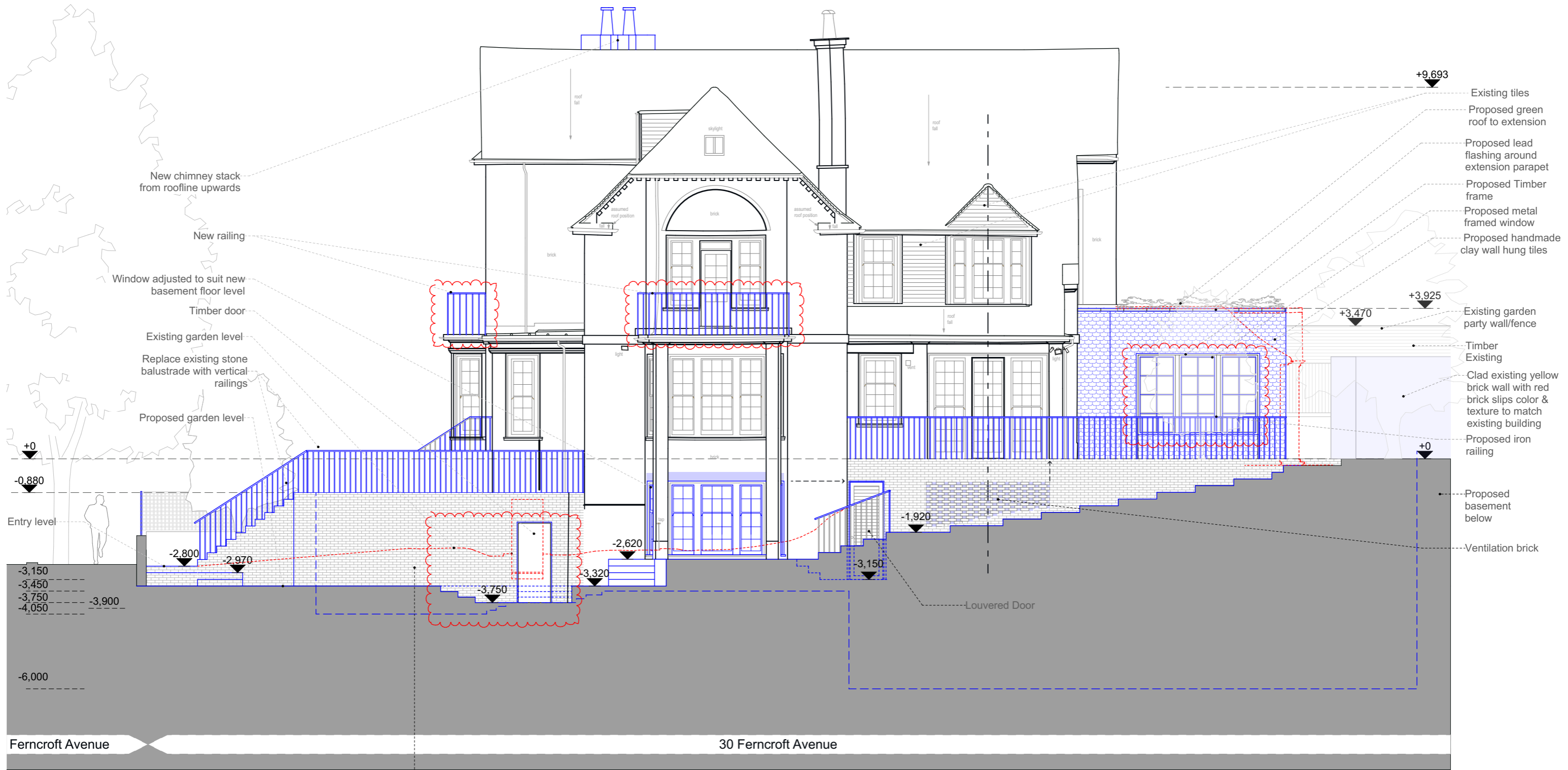
Front Side Elevation - East - towards Hollycroft Avenue
