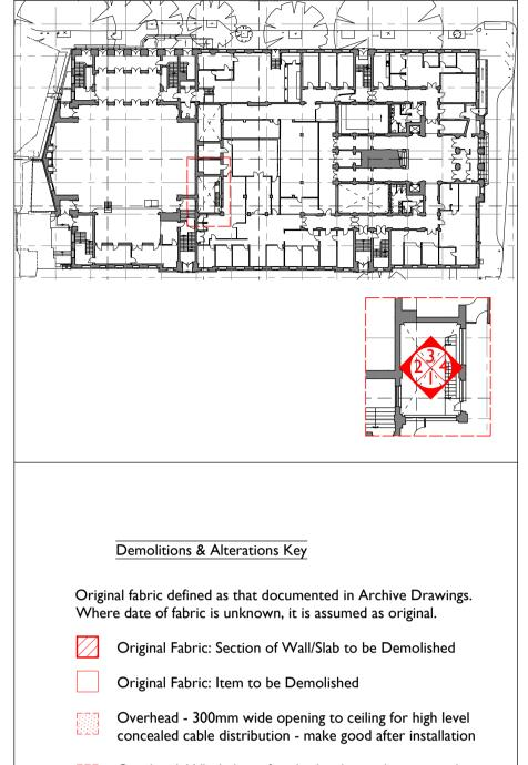
Overhead: Whole bay of vaulted ceiling to be removed for cabling distribution and reinstated
