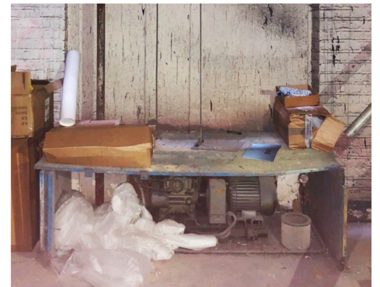
07 Winch to be retained and encased in clear box
